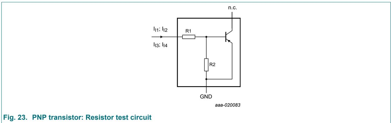
Fig. 23. PNP transistor: Resistor test circuit
