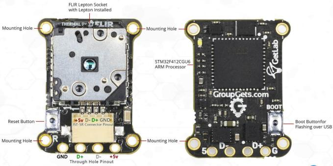
•PureThermal Mini Pro JST-SR supports all FLIR Lepton 2.x - 3.x cores with and without radiometry
