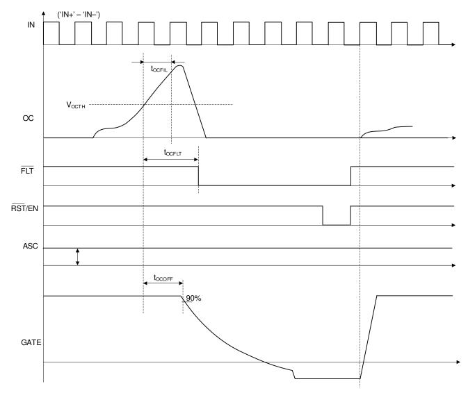
Figure 38. ASC Protection with OC Fault
