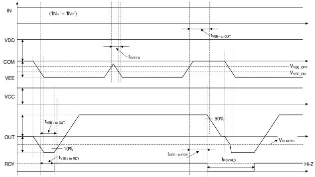
Figure 34. VEE UVLO Protection Timing Diagram
