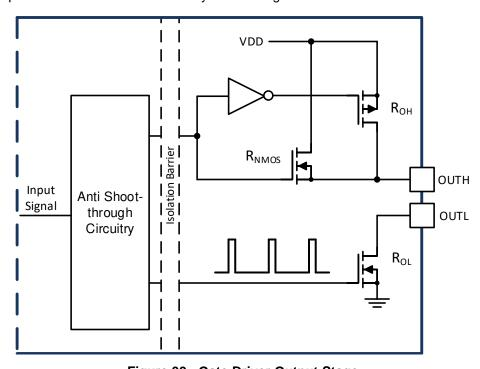
Figure 39. Gate Driver Output Stage
