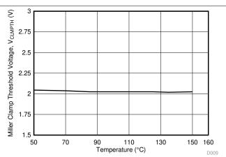
Figure 21. V<sub>CLMPTH</sub> Miller Clamp Threshold Voltage vs. Temperature
