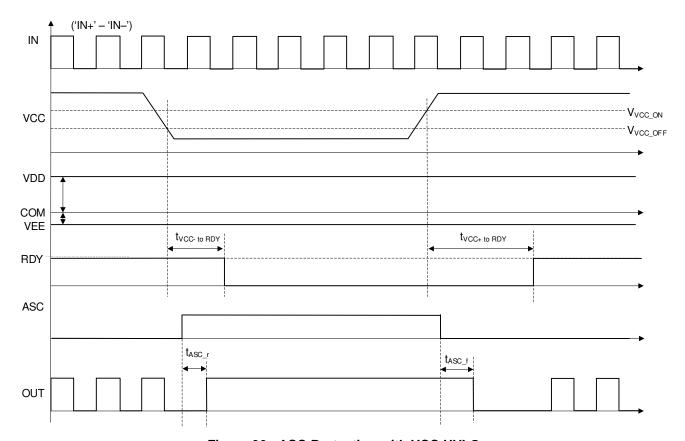
Figure 36. ASC Protection with VCC UVLO
