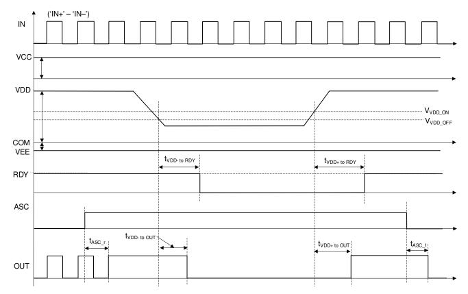
Figure 37. ASC Protection with VDD UVLO
