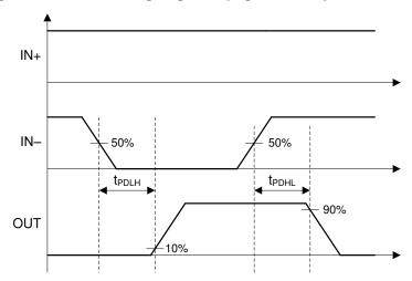
Figure 26. Inverting Logic Propagation Delay Measurement
