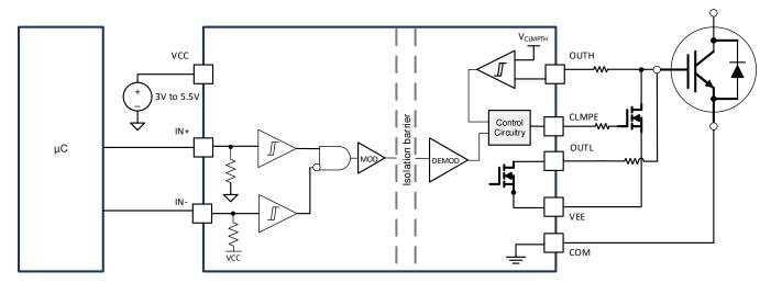
Figure 50. External Active Miller Clamp Configuration
