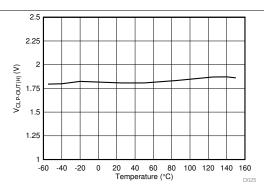
Figure 19. V<sub>CLP-OUT(H)</sub> Short Circuit Clamping Voltage vs. Temperature
