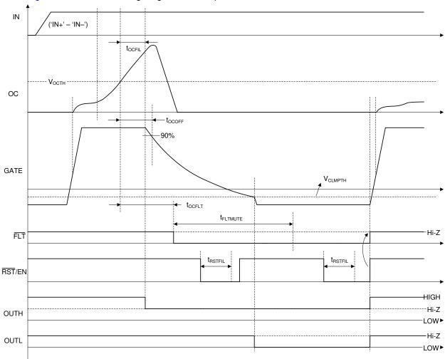
Figure 35. OC Protection with Soft Turn-OFF
