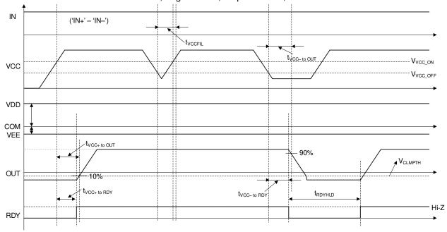
Figure 32. VCC UVLO Protection Timing Diagram
