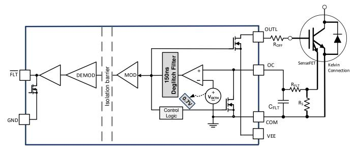
Figure 51. Overcurrent and Short Circuit Protection Based on IGBT Module with SenseFET
