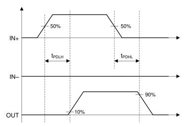
Figure 25. Non-inverting Logic Propagation Delay Measurement
