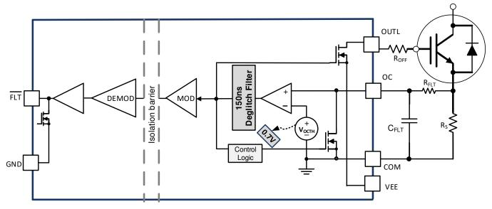
Figure 43. Overcurrent and Short Circuit Protection
