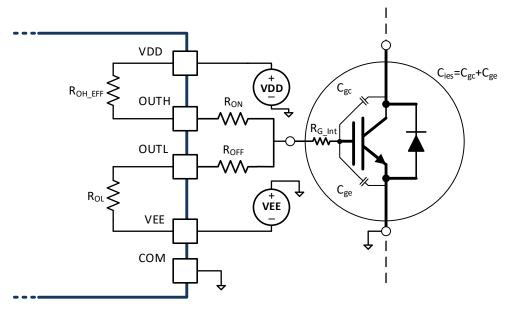
Figure 48. Output Model for Calculating Peak Gate Current
