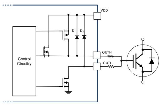
Figure 41. Short Circuit Clamping
