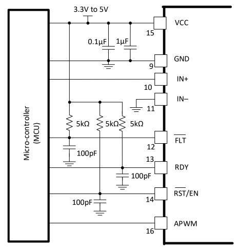
Figure 46. FLT, RDY and RST/EN Pins Circuitry
