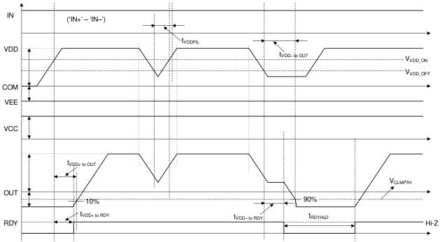
Figure 33. VDD UVLO Protection Timing Diagram
