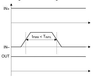
Figure 28. IN+ OFF Deglitch Filter
