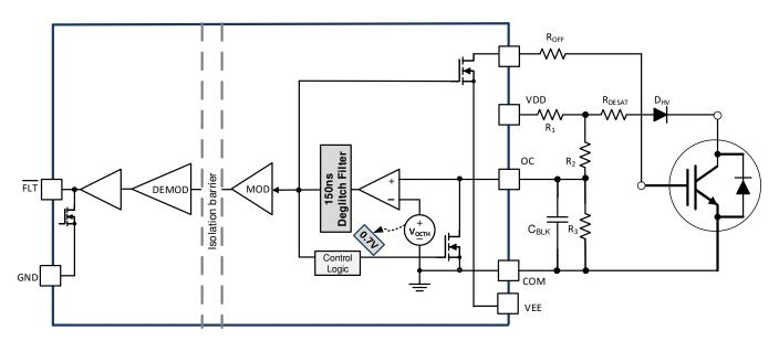
Figure 52. Overcurrent and Short Circuit Protection Based on Desaturation Circuit
