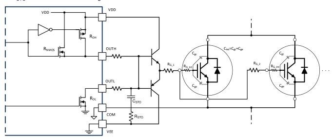
Figure 54. Current Buffer for Increased Drive Strength
