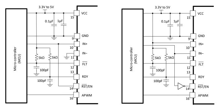
Figure 47. Automatic Reset Control
