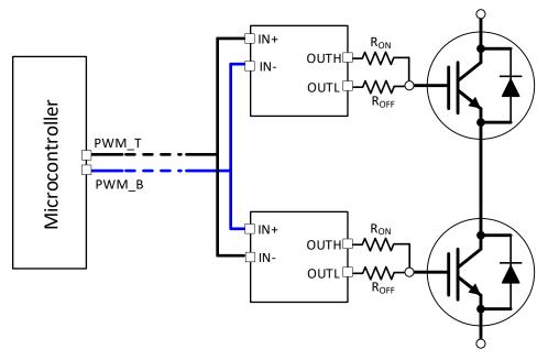
Figure 45. PWM Interlock for a Half Bridge
