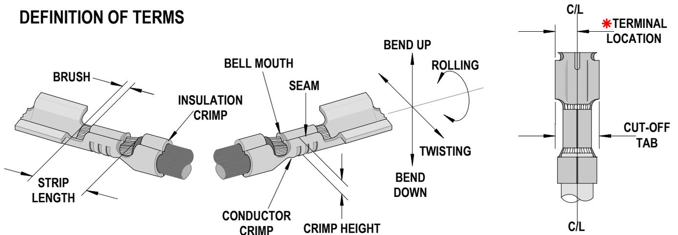
\* Terminal is to be centrally located between the two (2) cut-off tab edges by one half of the total cut-off tab tolerance.
