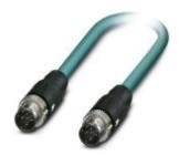
Network cable, Ethernet CAT5 (100 Mbps), 4-position, PUR, water blue RAL 5021, shielded, Plug straight M12 SPEEDCON / IP67, coding: D, on Plug straight M12 SPEEDCON / IP67, coding: D, cable length: 3 m
