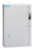
Non-reversing motor starter, Size 3, Three phase full voltage, Solid-state overload relay, OLR amp range 25-100A, 24VAC 50-60Hz coil, Combination type, 125A circuit breaker, Enclosure NEMA type 4/12, Water/dust tight for outdoors, Extra-wide enclosure
