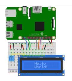
Pi 5V to LCD pin 2, 15, and one side of the potentiometer.
