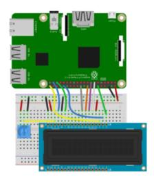
Pi 5V to LCD pin 2, 15, and one side of the potentiometer.
