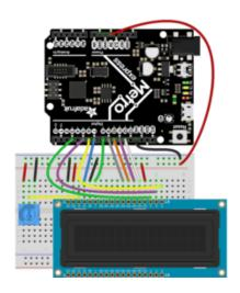
Board 5V to LCD pin 2, 15, and one side of the potentiometer.
