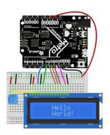
Board 5V to LCD pin 2 and one side of the potentiometer.
