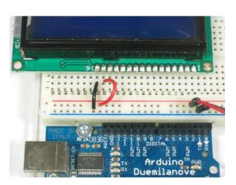
Next we'll connect up the backlight for the LCD. Connect pin 16 to ground and pin 15 to +5V. On the vast majority of LCDs (including ones from Adafruit) the LCD includes a series resistor for the LED backlight.
