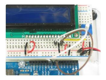
Next is the EN pin #6, we'll use a white wire to connect it to Arduino digital #8.
