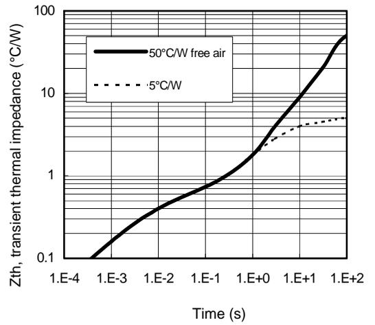
**Figure 15 – Transient thermal impedance ( $^{\circ}\text{C}/\text{W}$ ) Vs time (s)**
