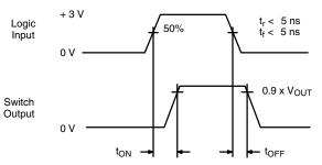
Logic "1" = Switch On Logic input waveforms inverted for switches that have the opposite logic sense.
