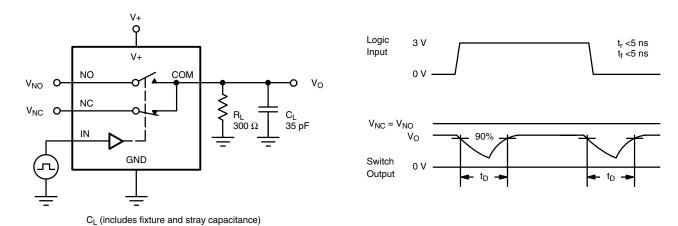
Figure 2. Break-Before-Make Interval
