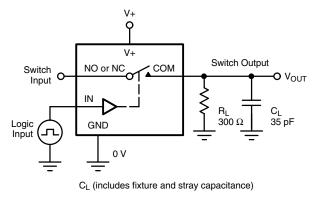
$$V_{OUT} = V_{COM} \left( \frac{R_L}{R_L + R_{ON}} \right)$$
