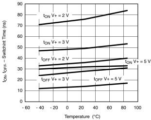
Switching Time vs. Temperature and Supply Voltage
