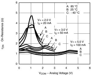
r<sub>ON</sub> vs. V<sub>COM</sub> and Supply Voltage
