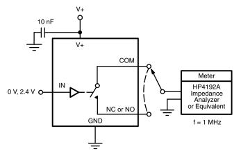
Figure 5. Channel Off/On Capacitance
