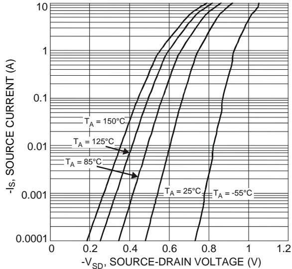
Fig. 7 Reverse Drain Current vs. Source-Drain Voltage
