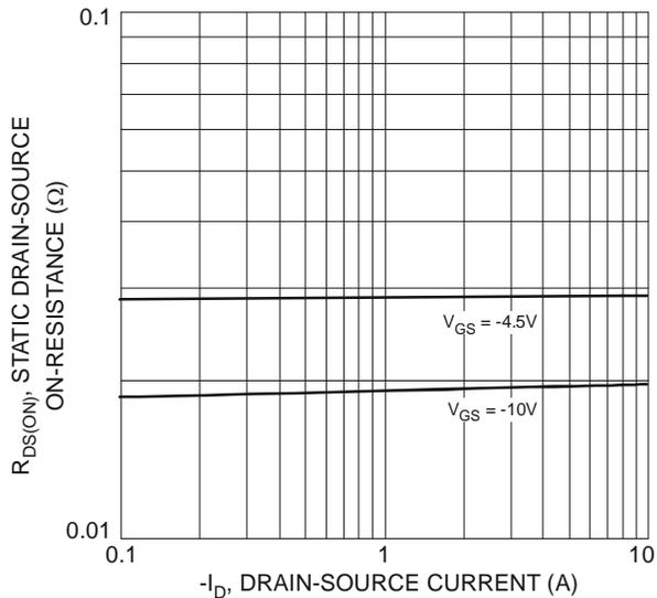
Fig. 3 On-Resistance vs. Drain Current & Gate Voltage
