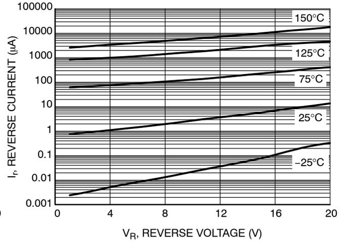
Figure 2. Leakage Current
