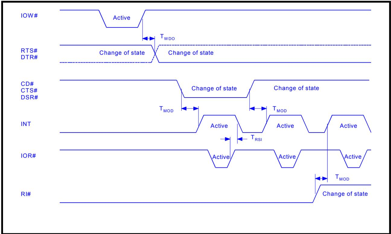
FIGURE 16. 16 MODE (INTEL) DATA BUS READ TIMING
