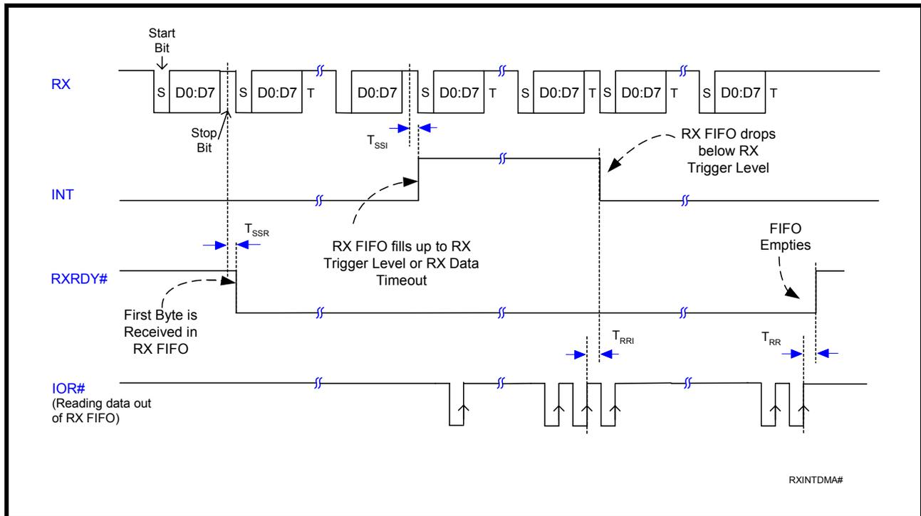
FIGURE 23. RECEIVE READY & INTERRUPT TIMING [FIFO MODE, DMA ENABLED] FOR CHANNELS A & B
