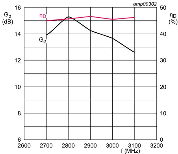
$V_{DS} = 32\text{ V}; I_{Dq} = 400\text{ mA}; P_L = 425\text{ W}; t_p = 300\text{ }\mu\text{s}; \delta = 10\text{ }\%$
