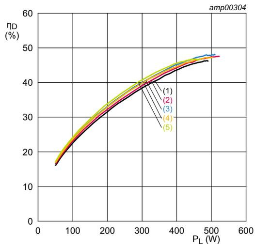
$V_{DS} = 32\text{ V}; I_{Dq} = 400\text{ mA}; t_p = 300\text{ }\mu\text{s}; \delta = 10\text{ }\%$
