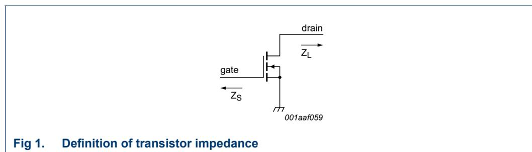
Fig 1. Definition of transistor impedance
