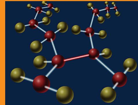
TE pioneered cross-linked insulation for wire and cable, initially for the aerospace industry. To achieve cross-linking, a polymer product is exposed to high-energy radiation. This is generally done by exposure to high-energy electron beta radiation using an electron beam.
