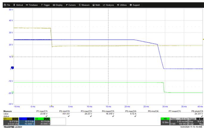
**Hold Up/Interruption Time: Measured hold up time with 24Vo/300W**
