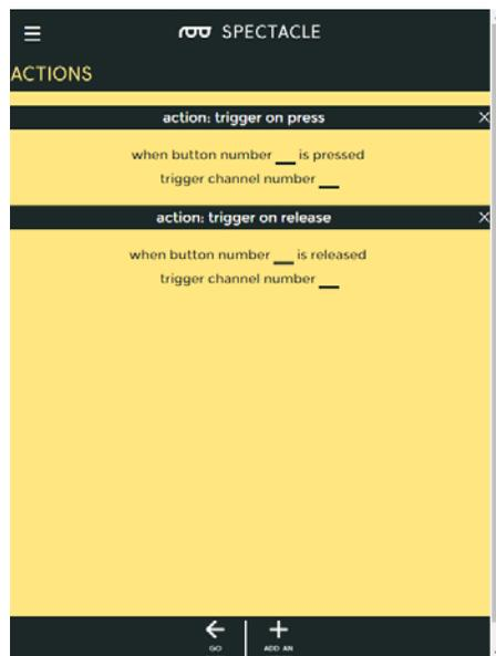
Here are the settings you'll want to put into place for this project. You can see that the "Action on Press" is tied to channel 0, and we're using button 8 (the onboard button) as the input signal. "Action on Release" is tied to channel 1, and also to button 8.
