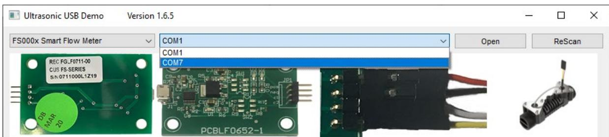
In the case above the hardware was assigned to COM7. Select the new port that was added to Establish communication between the GUI and the pcb.
