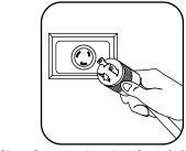
AC Input Connection: Insert L6-20P twist-lock plug into compatible L6-20R utility, generator or UPS outlet. For international applications, connect user-supplied power cord with region-specific plug to C20 power inlet.
