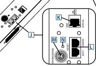
Network Interface: Connect to Ethernet for remote monitoring via SNMP, Web or Telnet. Add optional ENVIROSENSE accessory for temperature/humidity monitoring and dry contact interface.
