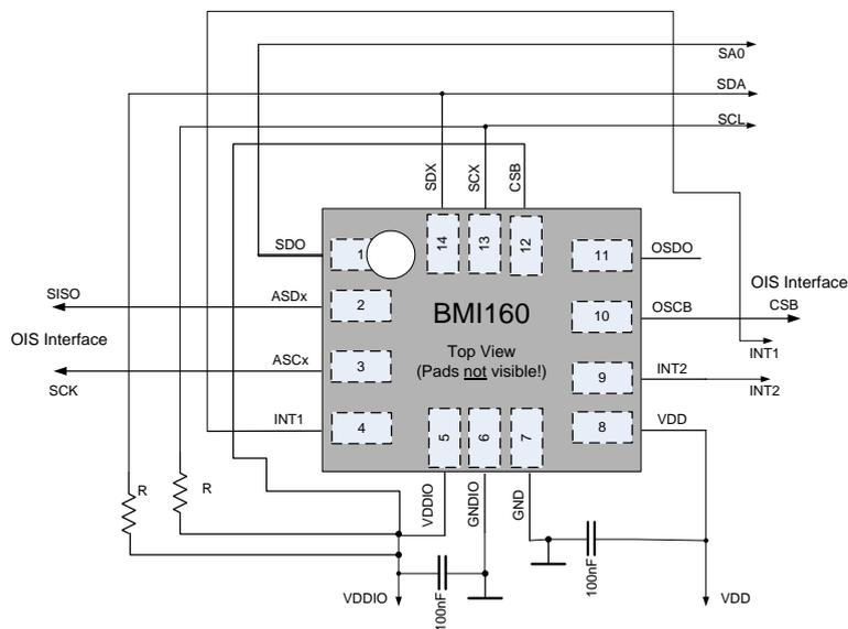
Figure 40: Using I<sup>2</sup>C and 3-wire SPI as OIS interface
