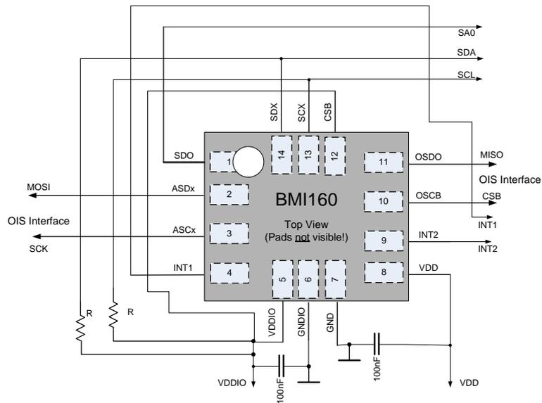
Figure 39: Using I<sup>2</sup>C and 4-wire SPI as OIS interface
