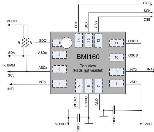
Figure 37: Using SPI 3-wire and the magnetometer interface
