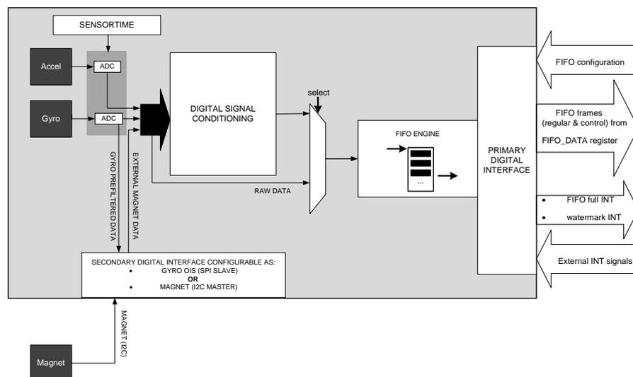
Figure 3: Block diagram of FIFO data path
