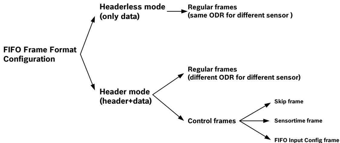
Figure 4: FIFO frame configurations
