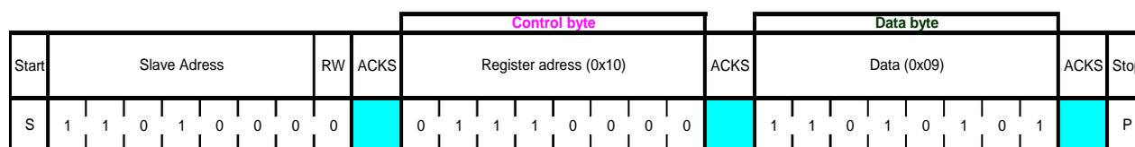
Figure 28: I<sup>2</sup>C write
