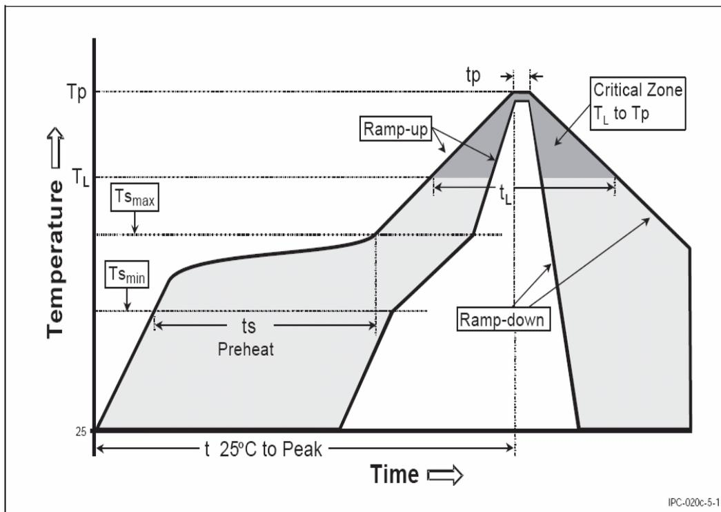
Figure 45: Soldering profile
