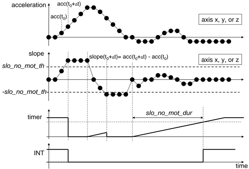
Figure 17: Signal timings no motion interrupt
