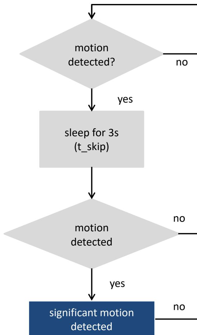
Figure 6: Block diagram of significant motion interrupt algorithm
