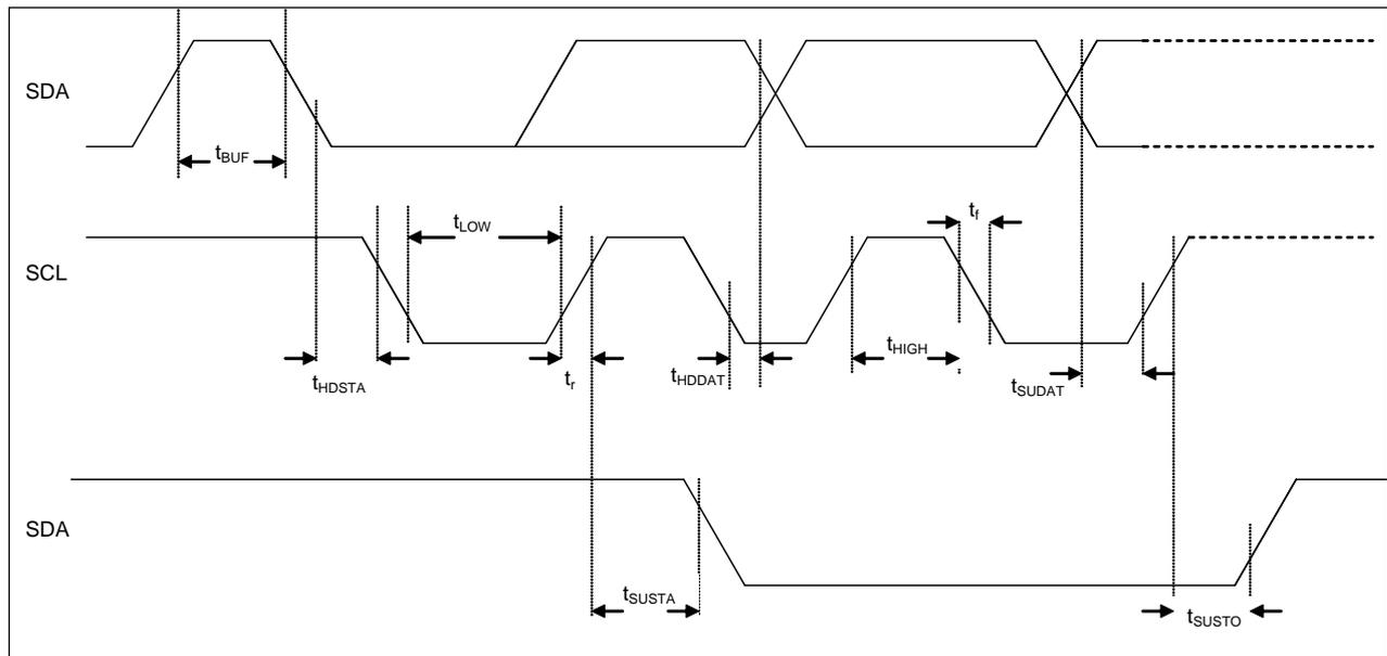
Figure 27: I<sup>2</sup>C timing diagram
