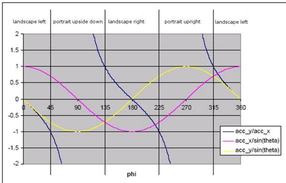
Figure 9: Angle-to-Orientation Mapping
