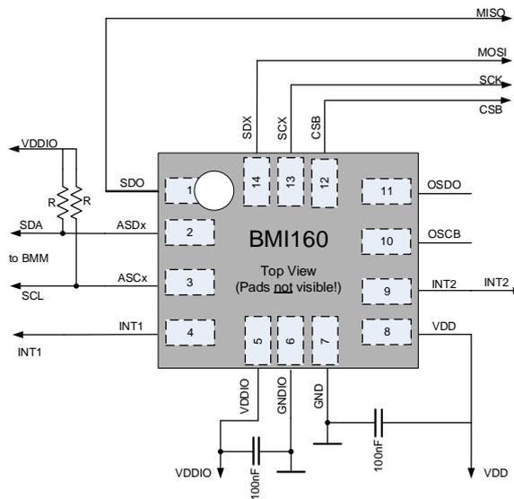
Figure 36: Using SPI 4-wire and the magnetometer interface
