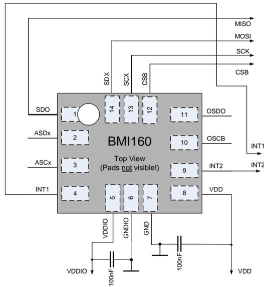
Figure 35: Only SPI 4-wire as primary interface
