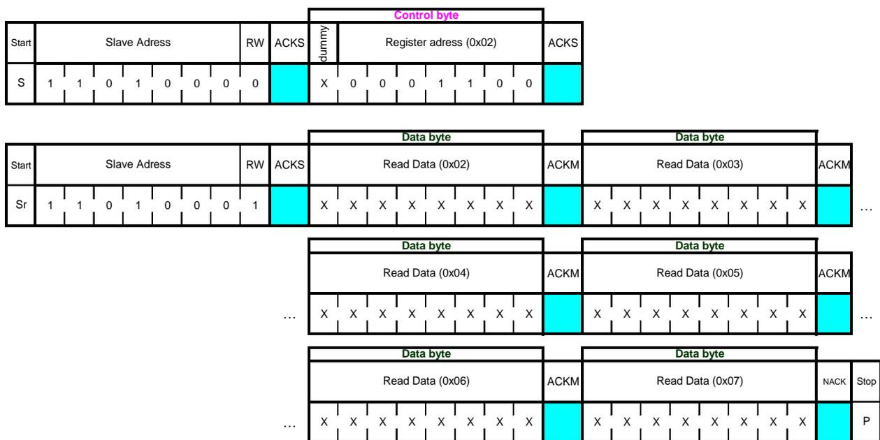
Figure 29: I<sup>2</sup>C multiple read
