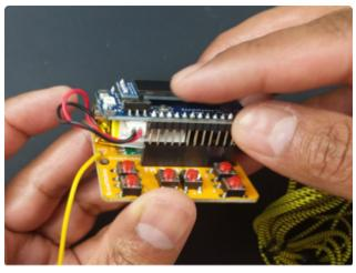
Connect the Azul Bluetooth board to the FM board as shown in the picture. Ensure the headers line up correctly before pressing the 2 boards together.
