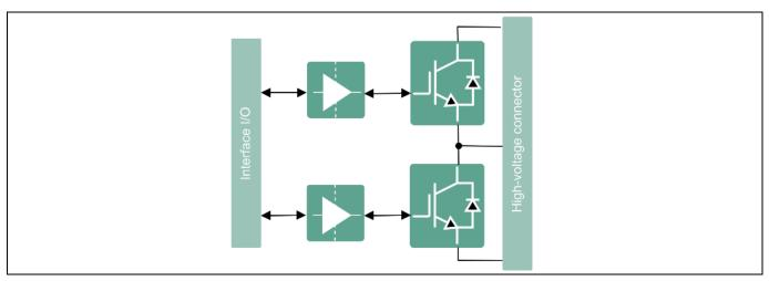
Figure 2 Eval-1ED3321MC12N evaluation board block diagram
