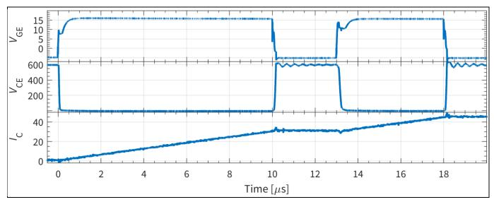
Figure 3 Eval-1ED3321MC12N – Double-pulse test of the low side IGBT with a 200 μH load
