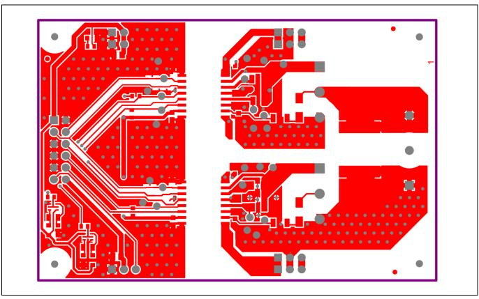
Figure 11 Eval-1ED3321MC12N - PCB top layer view
