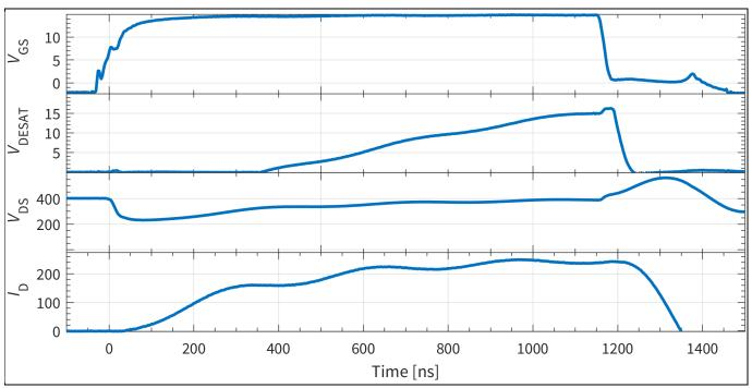
Figure 6 Eval-1ED3321MC12N – Turn-off of Type I short-circuit with CoolSiC™ without desaturation capacitor
