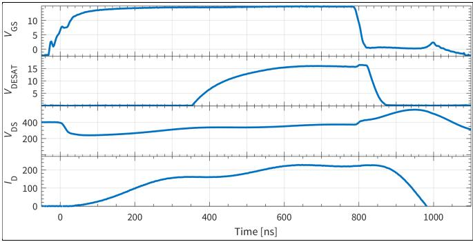
Figure 8 Eval-1ED3321MC12N – Turn-off of Type I short-circuit with CoolSiC™ without desaturation capacitor, 60 V SOD523 for D5 and D15 and 3 kΩ for R9 and R19
