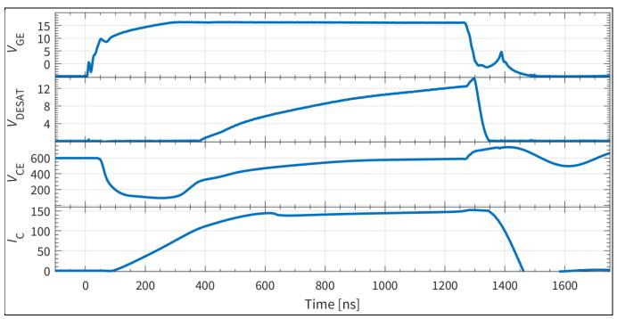
Figure 4 Eval-1ED3321MC12N - Turn-off of Type I short-circuit
