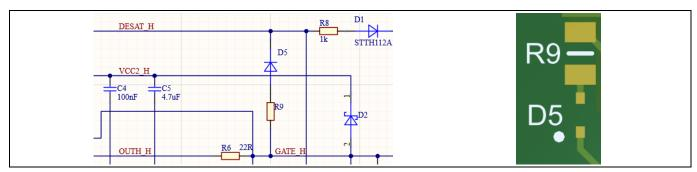
Figure 7 DESAT pin overdrive circuit
