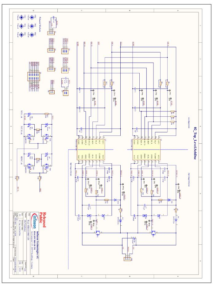
Figure 9 Eval-1ED3321MC12N - Schematic
