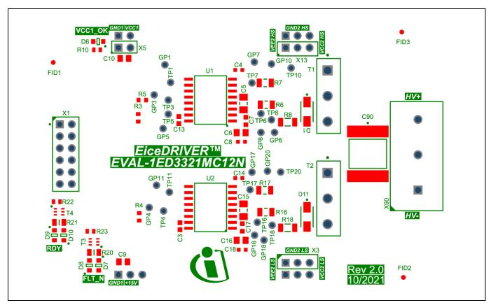
Figure 10 Eval-1ED3321MC12N - Assembly drawing top side
