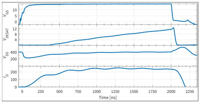
Eval-1ED3321MC12N - Turn-off of Type I short-circuit with CoolSiC™ and default board Figure 5 configuration
