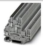
Double-level terminal block, Cross section: 0.14 mm² - 4 mm², AWG: 26 - 12, Connection type: Screw/plug-in connection, Width: 5.2 mm, Color: gray, Mounting type: NS 35/7,5, NS 35/15
