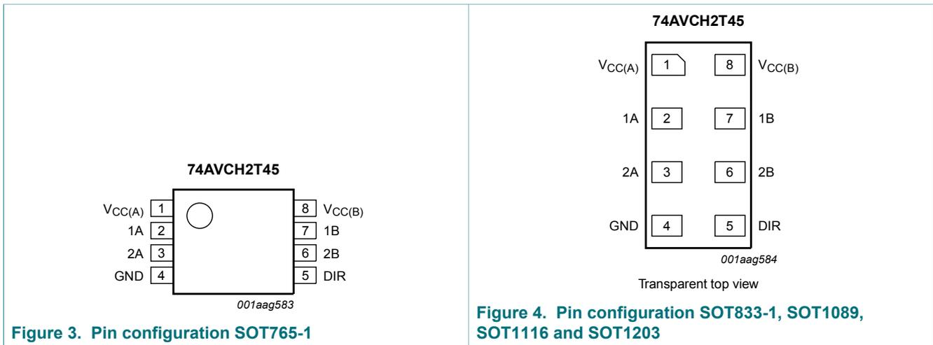
Figure 3. Pin configuration SOT765-1
