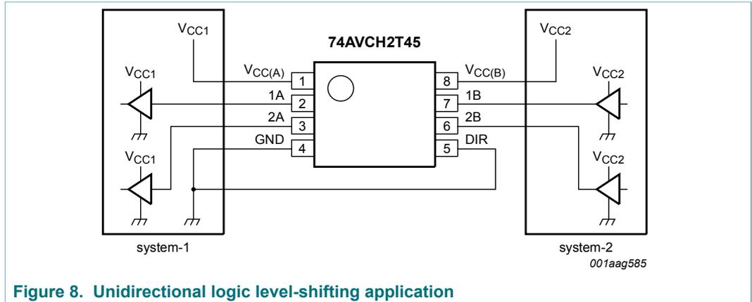
Figure 8. Unidirectional logic level-shifting application
