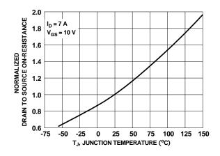
Figure 3. Normalized On-Resistance vs Junction Temperature
