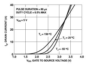
Figure 5. Transfer Characteristics
