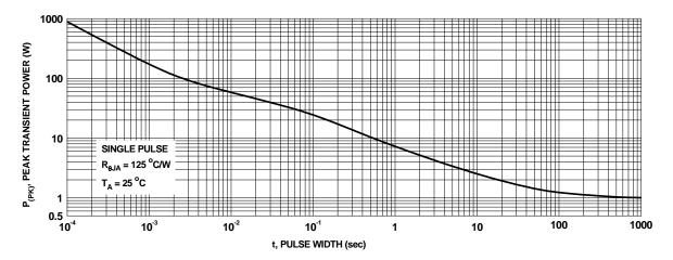
Figure 13. Single Pulse Maximum Power Dissipation
