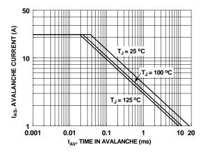
Figure 9. Unclamped Inductive Switching Capability
