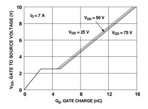
Figure 7. Gate Charge Characteristics
