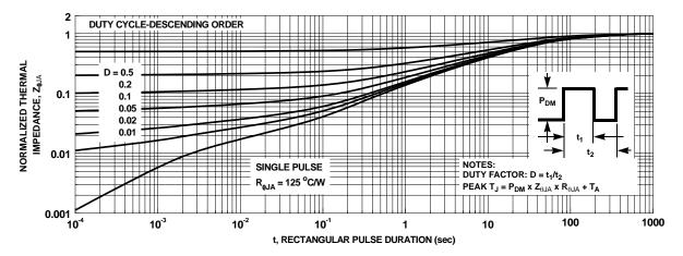
Figure 14. Junction-to-Ambient Transient Thermal Response Curve
