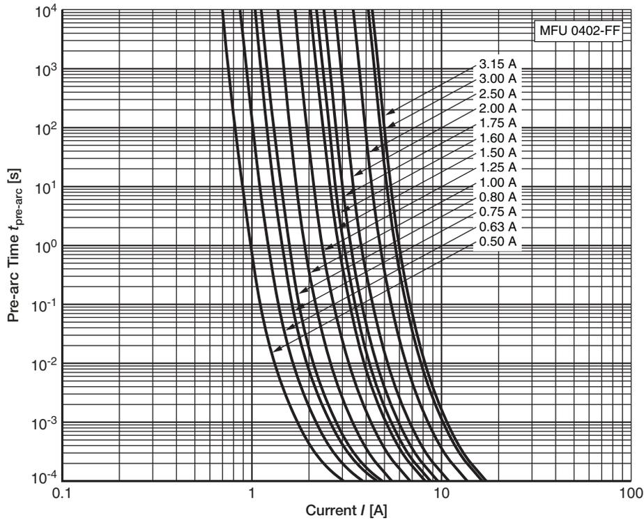
Typical  $t_{pre-arc}$  vs.  $I$  characteristic of MFU 0402 <sup>(1)</sup>
