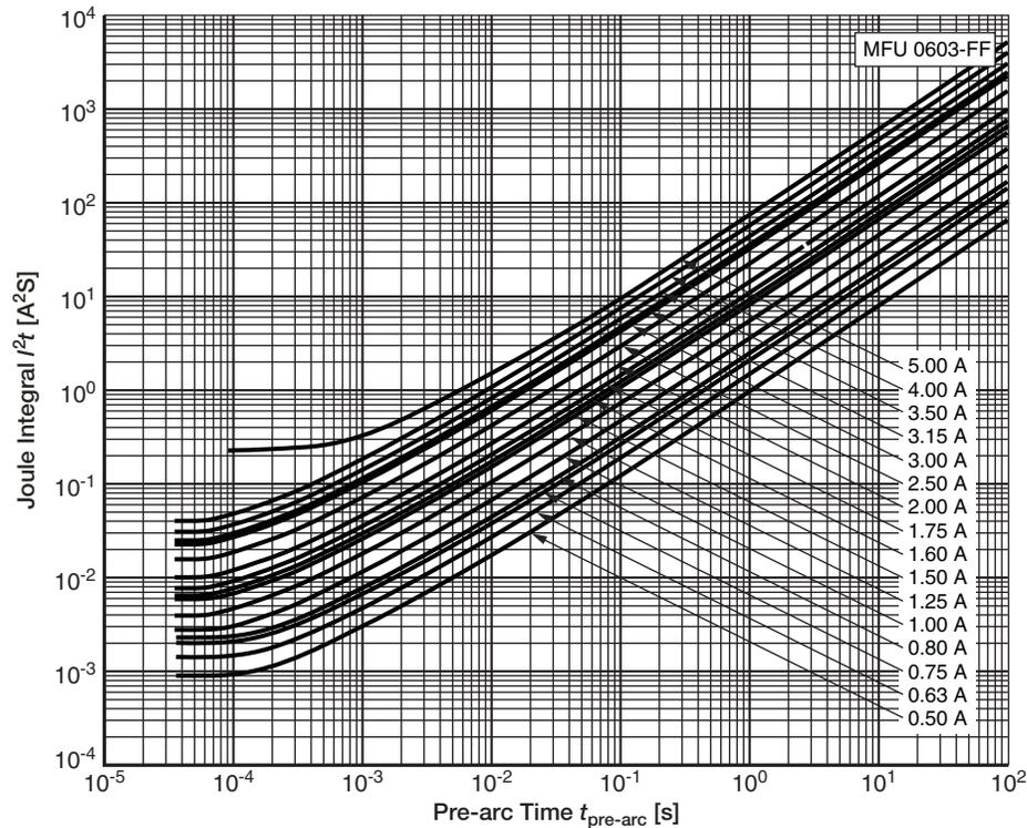
Typical  $I^2t$  vs.  $t_{pre-arc}$  characteristic of MFU 0603 <sup>(1)</sup>
