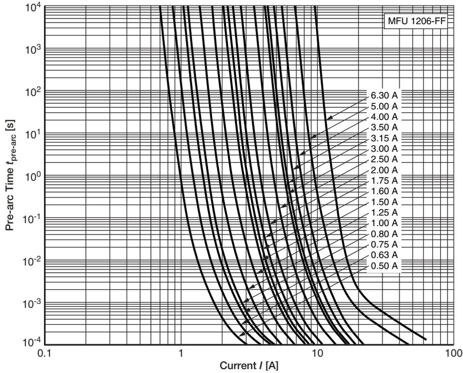
Typical  $t_{pre-arc}$  vs.  $I$  characteristic of MFU 1206 <sup>(1)</sup>
