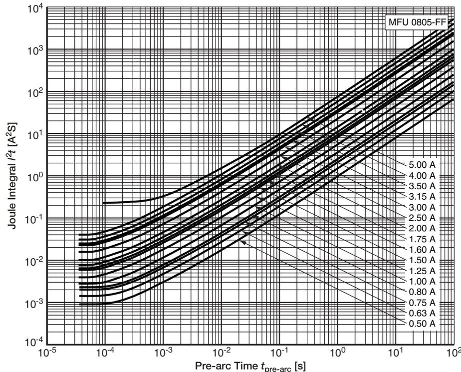
Typical  $I^2t$  vs.  $t_{pre-arc}$  characteristic of MFU 0805 <sup>(1)</sup>
