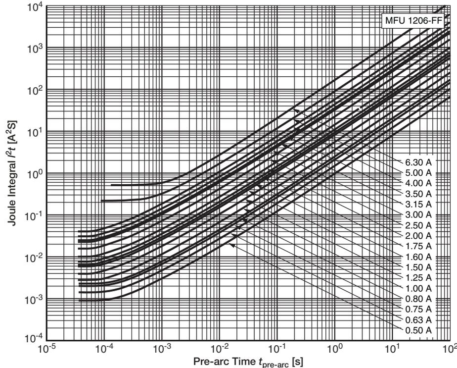
Typical  $I^2t$  vs.  $t_{pre-arc}$  characteristic of MFU 1206 <sup>(1)</sup>
