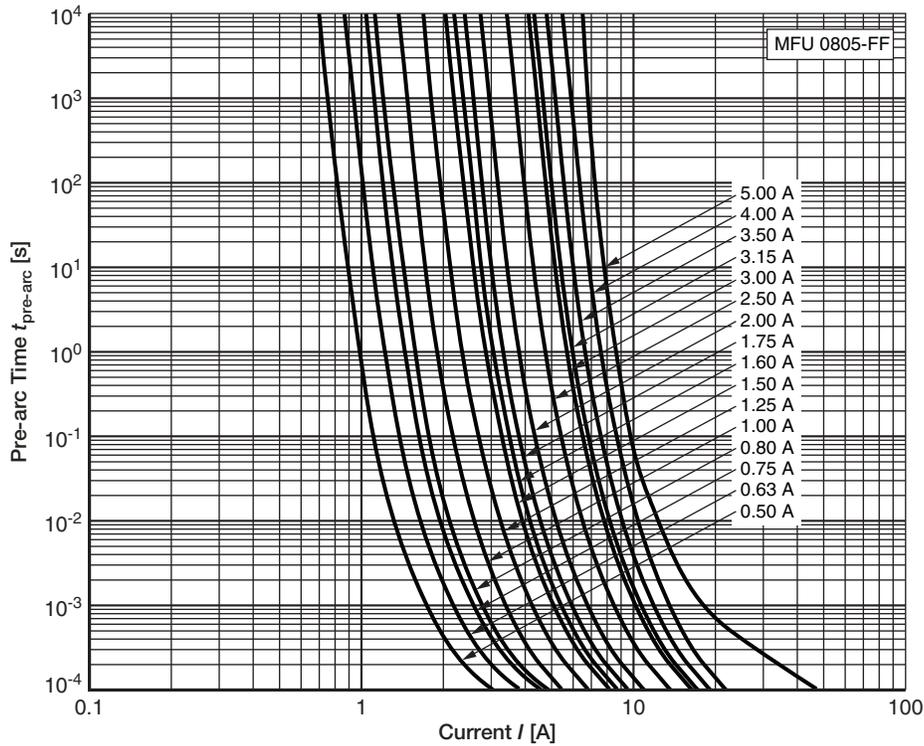
Typical  $t_{pre-arc}$  vs.  $I$  characteristic of MFU 0805 <sup>(1)</sup>
