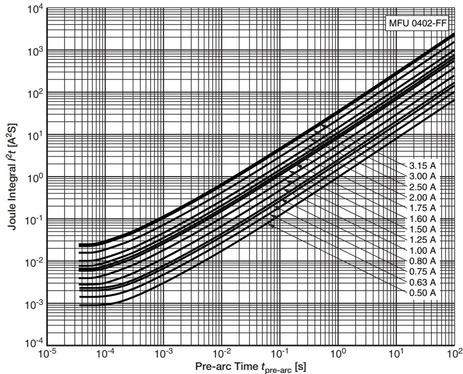
Typical  $I^2t$  vs.  $t_{pre-arc}$  characteristic of MFU 0402 <sup>(1)</sup>
