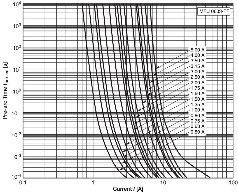
Typical  $t_{pre-arc}$  vs.  $I$  characteristic of MFU 0603 <sup>(1)</sup>
