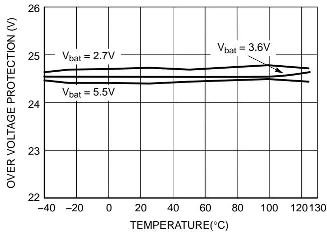
Figure 22. Overvoltage Protection
