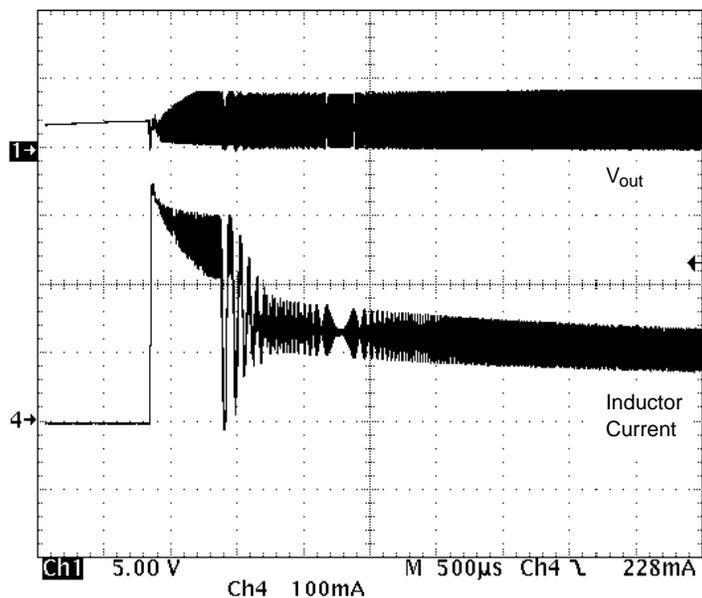
Conditions:  $V_{bat} = 3.6\text{ V}$ ,  $L_{out} = 22\ \mu\text{H}$ , 5 LED,  $I_{out} = 15\text{ mA}$
