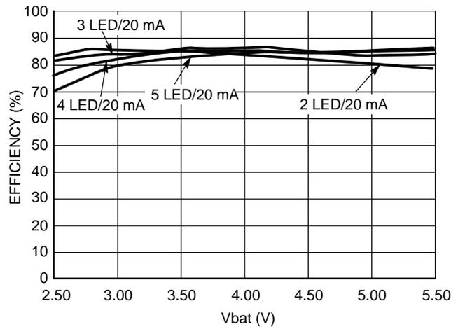
**Figure 13. Overall Efficiency vs. Power Supply –
