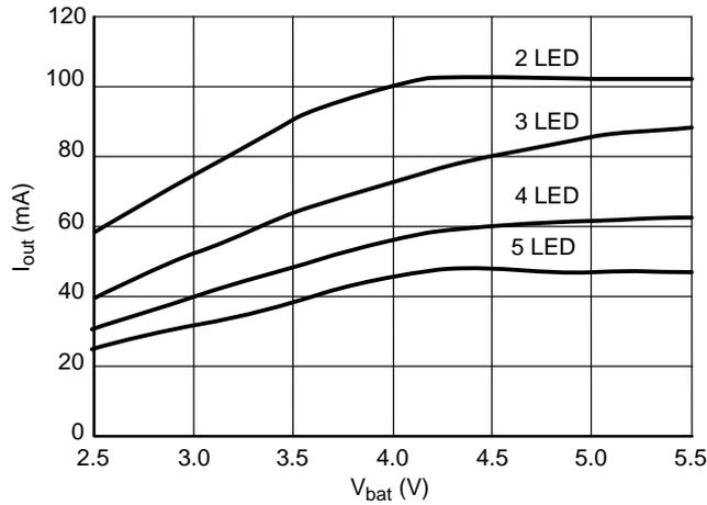
Test conditions: L = 22  $\mu$ H, R<sub>sense</sub> = 2.0  $\Omega$ , T<sub>amb</sub> = +25°C
