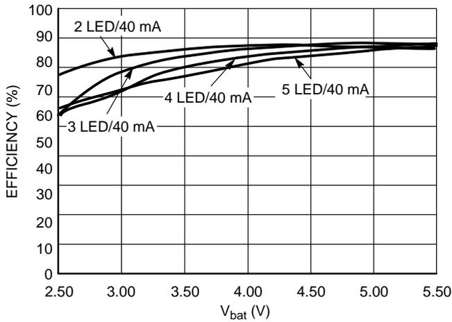
Figure 14. Overall Efficiency vs. Power Supply – I<sub>out</sub> = 40 mA, L = 22  $\mu$ H
