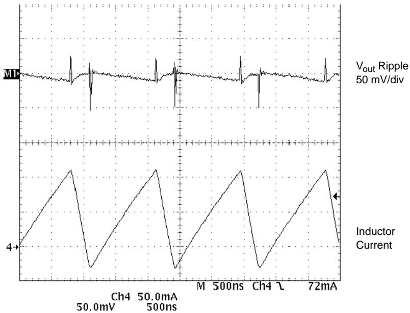
Conditions:  $V_{bat} = 3.6\text{ V}$ ,  $L_{out} = 22\ \mu\text{H}$ , 5 LED,  $I_{out} = 15\text{ mA}$
