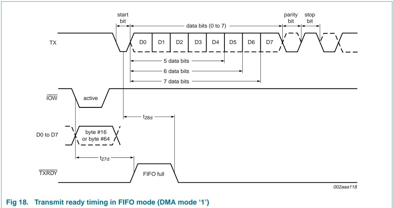
Fig 18. Transmit ready timing in FIFO mode (DMA mode '1')
