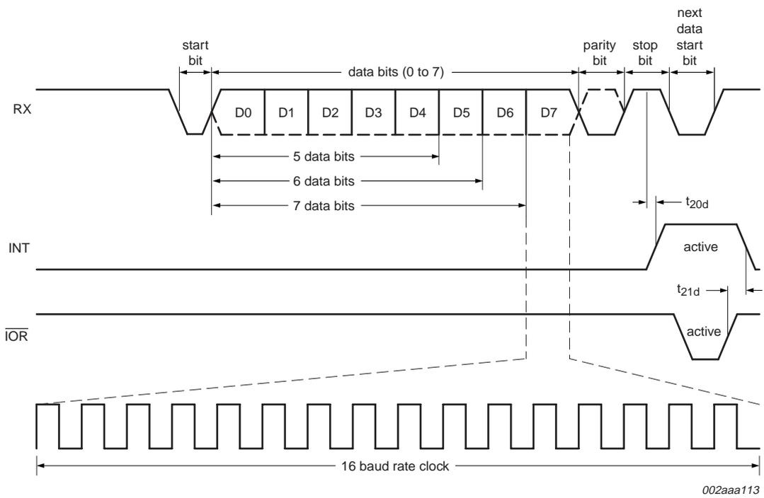
Fig 13. Receive timing
