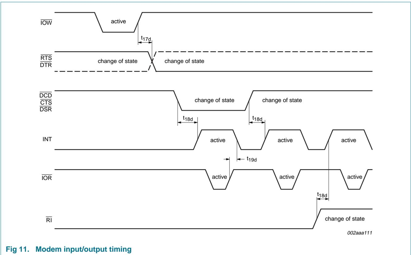
Fig 11. Modem input/output timing
