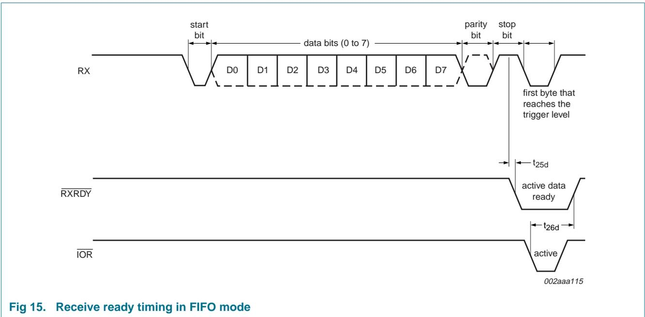
Fig 15. Receive ready timing in FIFO mode
