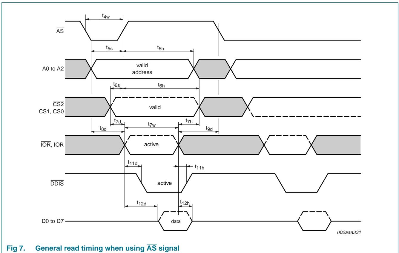
**Fig 7. General read timing when using  $\overline{\text{AS}}$  signal**
