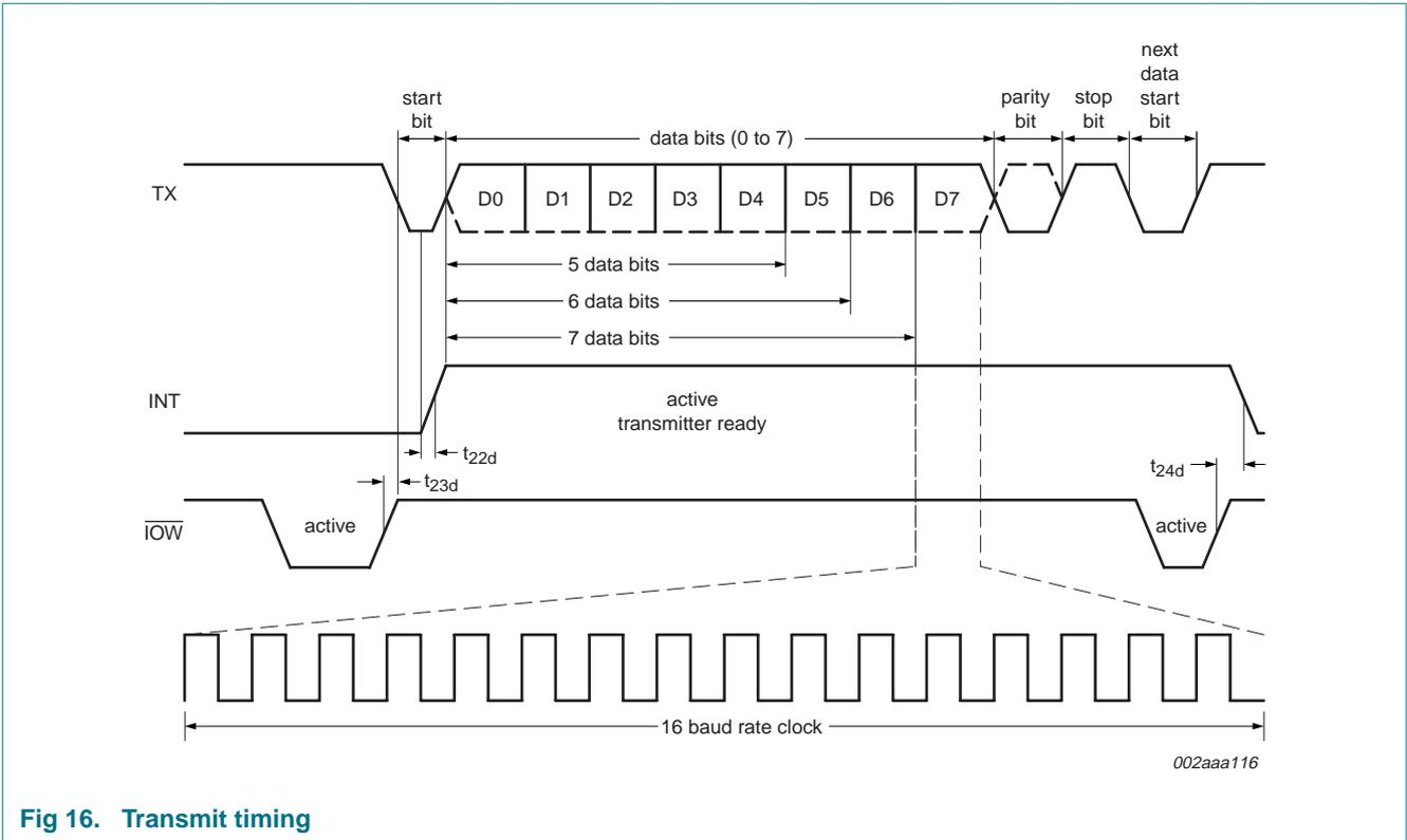
Fig 16. Transmit timing
