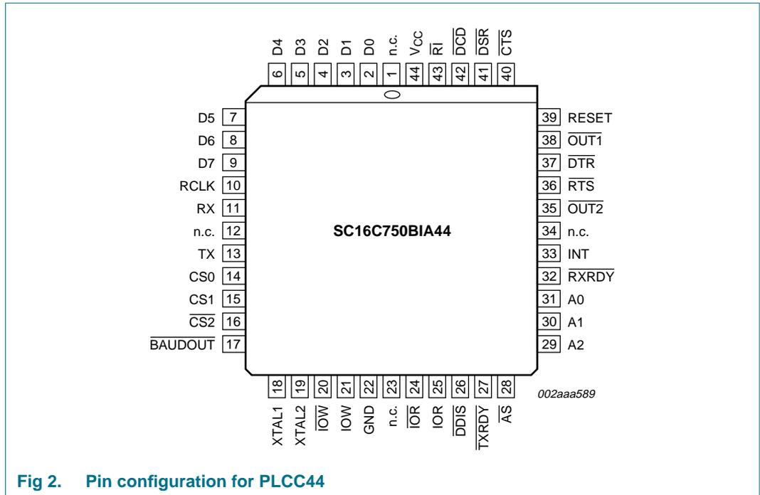
Fig 2. Pin configuration for PLCC44
