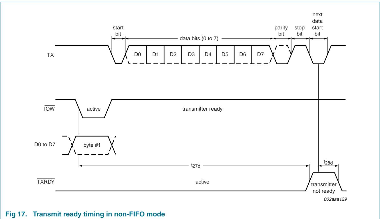
Fig 17. Transmit ready timing in non-FIFO mode
