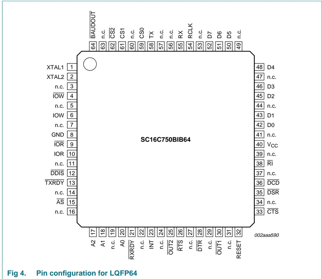
Fig 4. Pin configuration for LQFP64
