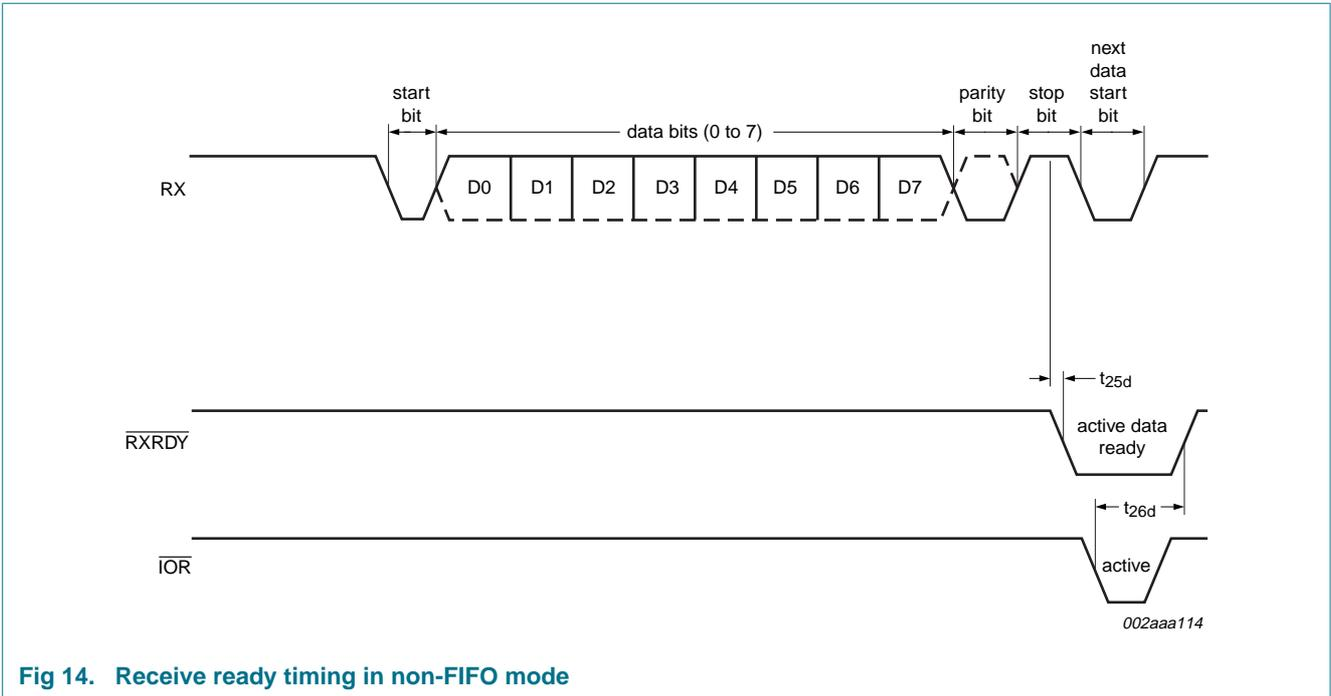
Fig 14. Receive ready timing in non-FIFO mode
