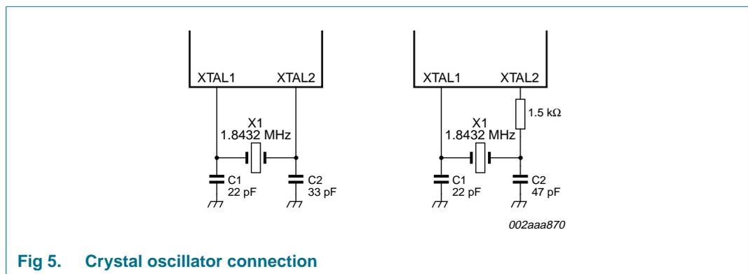
Fig 5. Crystal oscillator connection
