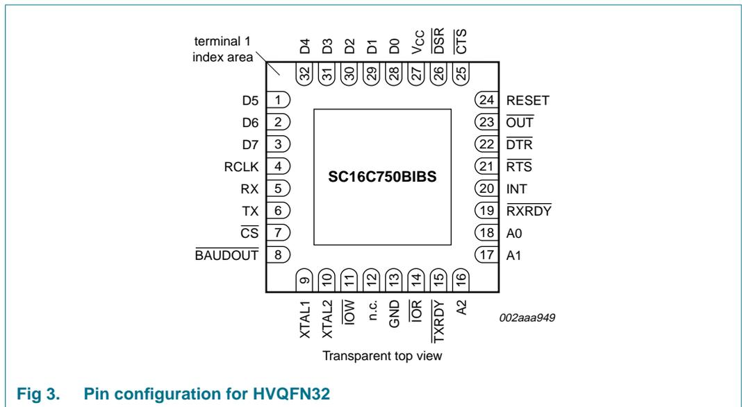
Fig 3. Pin configuration for HVQFN32
