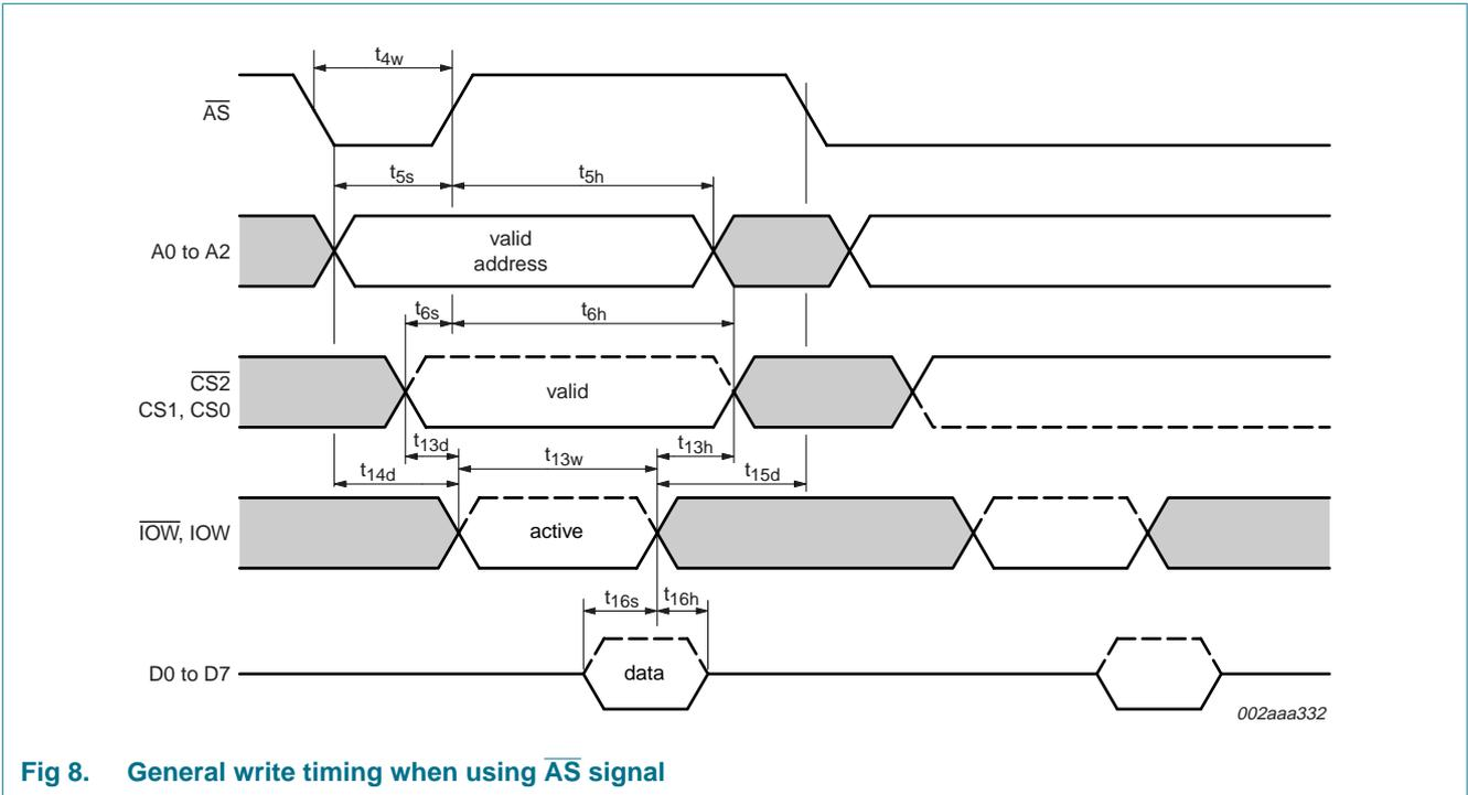
Fig 8. General write timing when using  $\overline{AS}$  signal
