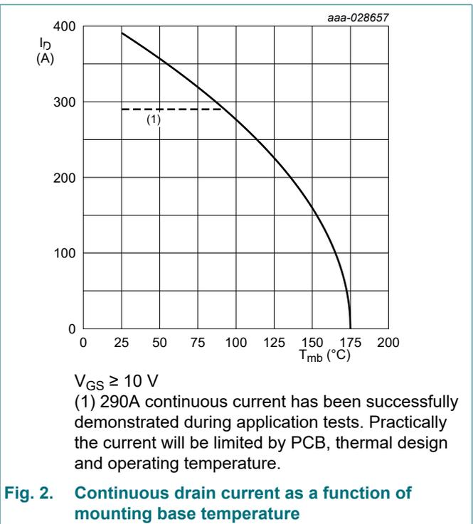
N-channel 40 V, 1 mΩ, 290 A standard level MOSFET in LPAK56E using NextPower-S3 Schottky-Plus technology
