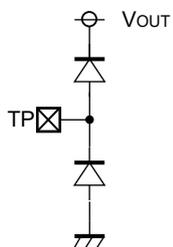
**TP Pin Equivalent Circuit Diagram
