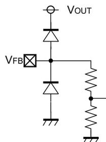
**VFB Pin Equivalent Circuit Diagram
