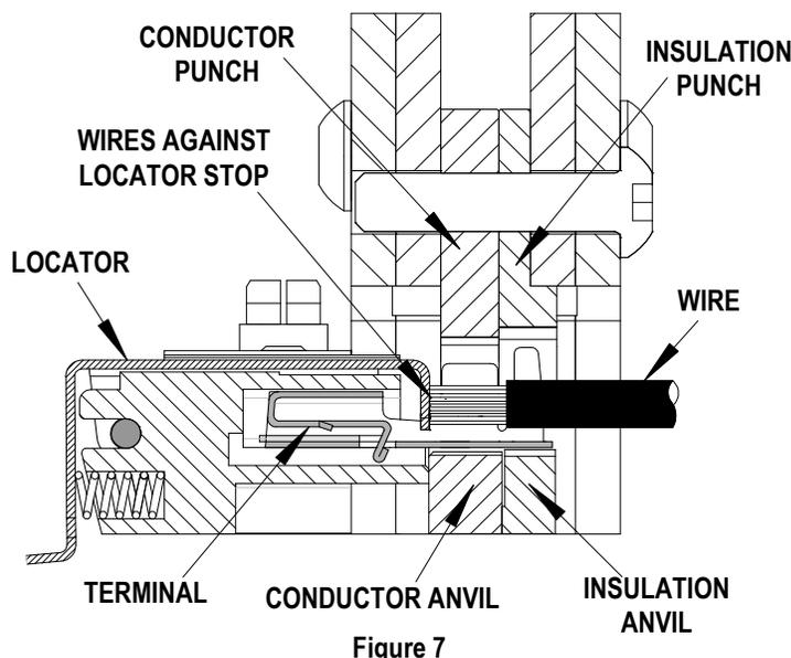
10. Remove the crimped terminal from the terminal locator by pressing down on the wire stop and gently pulling on the wire. The terminal locator can be in either position.
