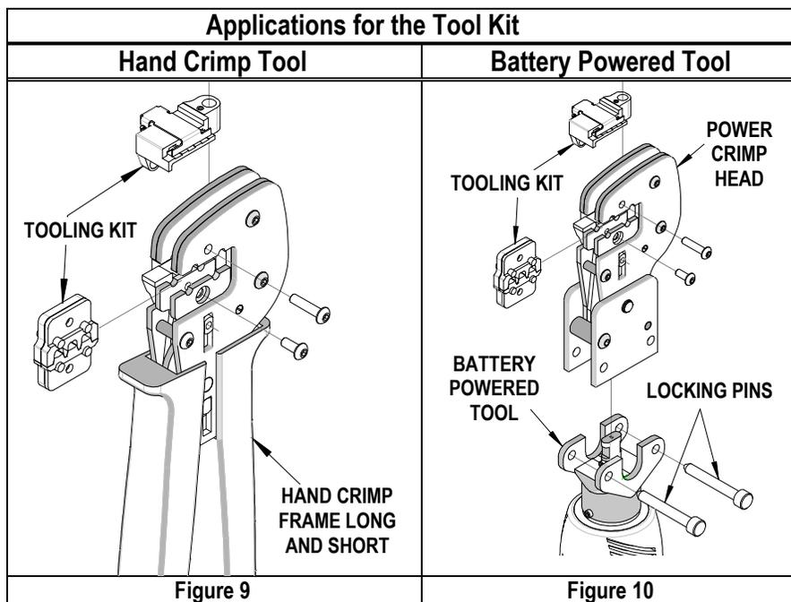
**WARNING:** NEVER operate service, install tool kits, or adjust the Power Crimp Head without proper instruction and without first reading and understanding the instructions in the proper Manual or Specification Sheet. See Chart above for the correct Manual or Specification Sheet.
