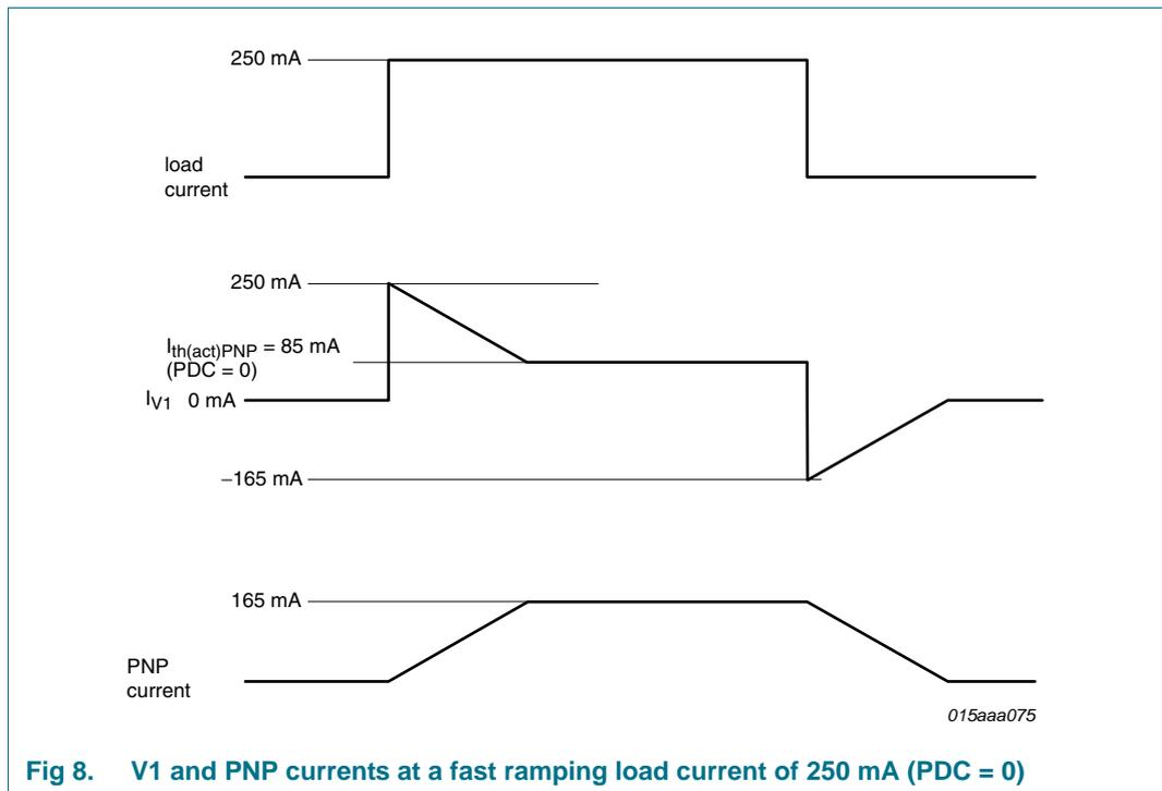
Fig 8. V1 and PNP currents at a fast ramping load current of 250 mA (PDC = 0)
