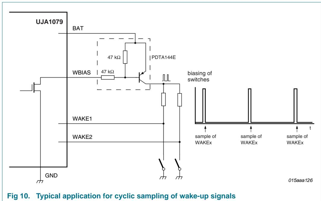
**Fig 10. Typical application for cyclic sampling of wake-up signals**
