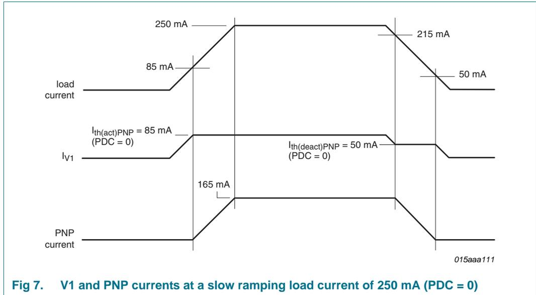
Fig 7. V1 and PNP currents at a slow ramping load current of 250 mA (PDC = 0)
