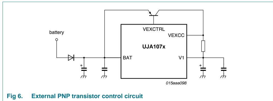
Fig 6. External PNP transistor control circuit
