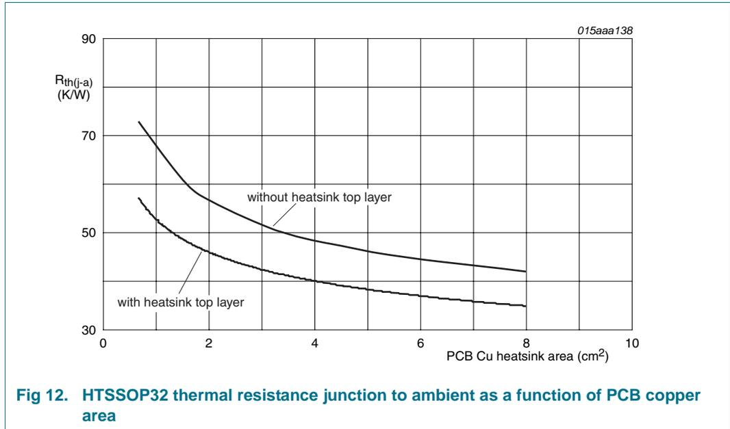
Fig 12. HTSSOP32 thermal resistance junction to ambient as a function of PCB copper area
