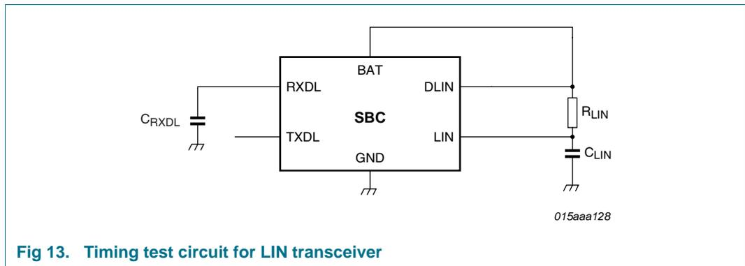
Fig 13. Timing test circuit for LIN transceiver
