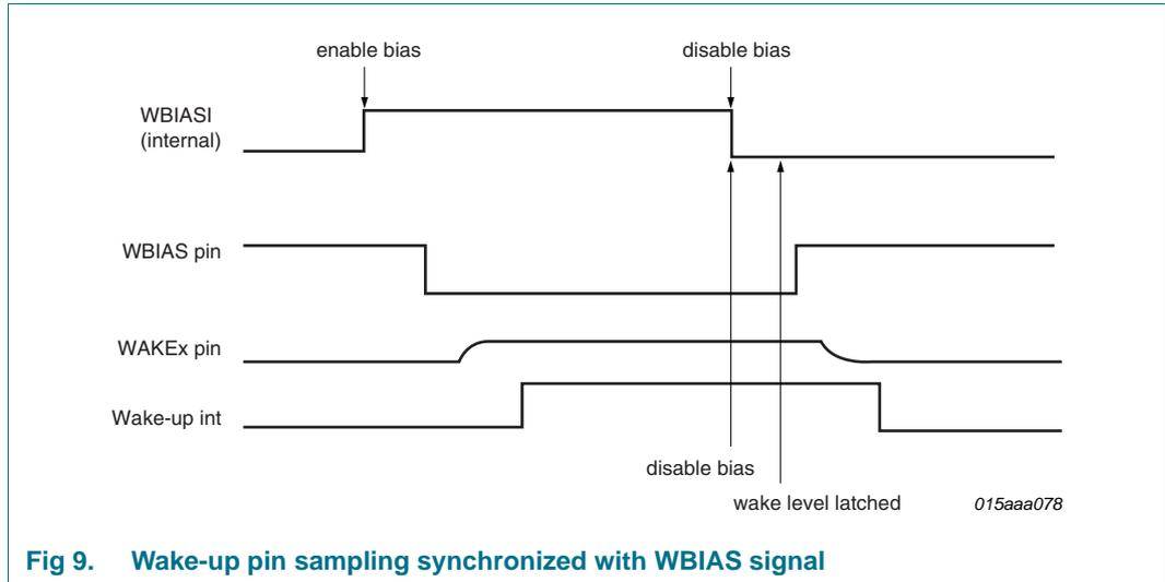
**Fig 9. Wake-up pin sampling synchronized with WBIAS signal**
