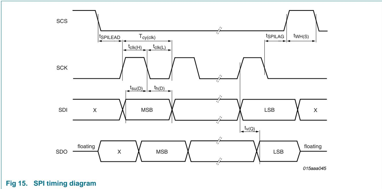
Fig 15. SPI timing diagram
