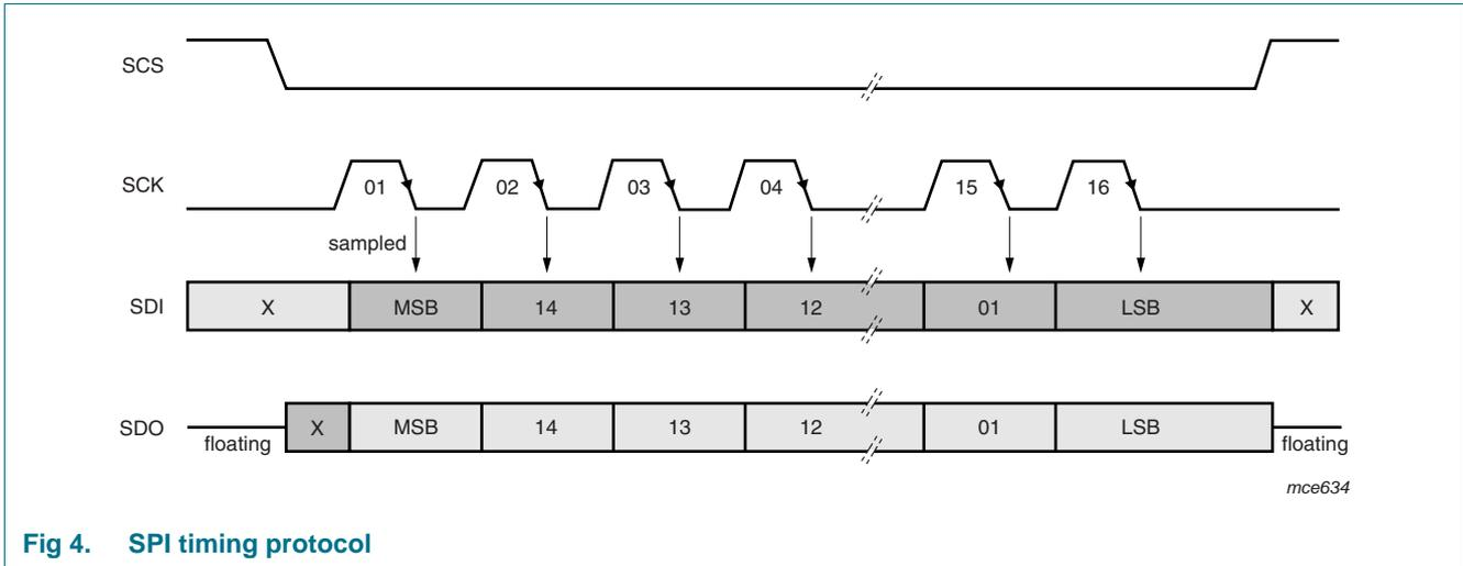
Fig 4. SPI timing protocol
