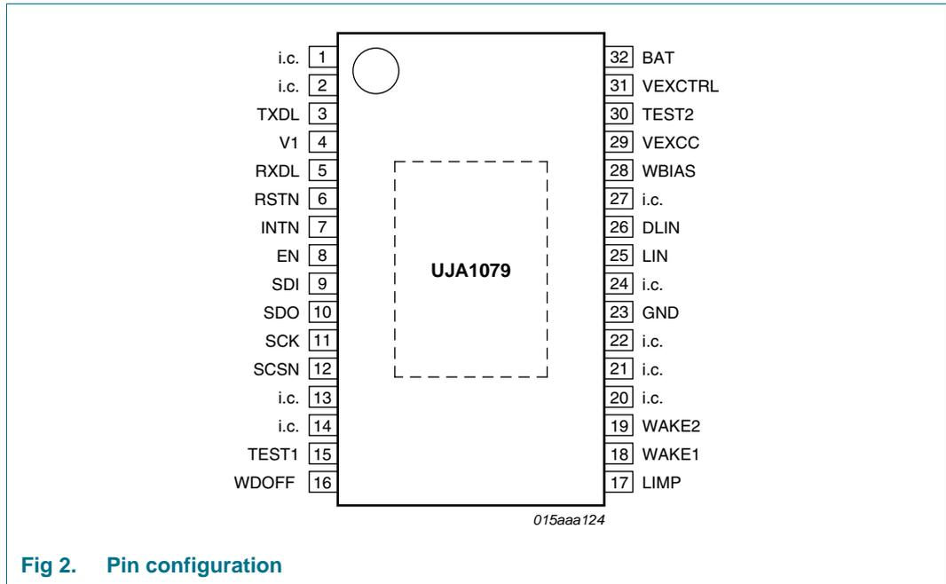
Fig 2. Pin configuration
