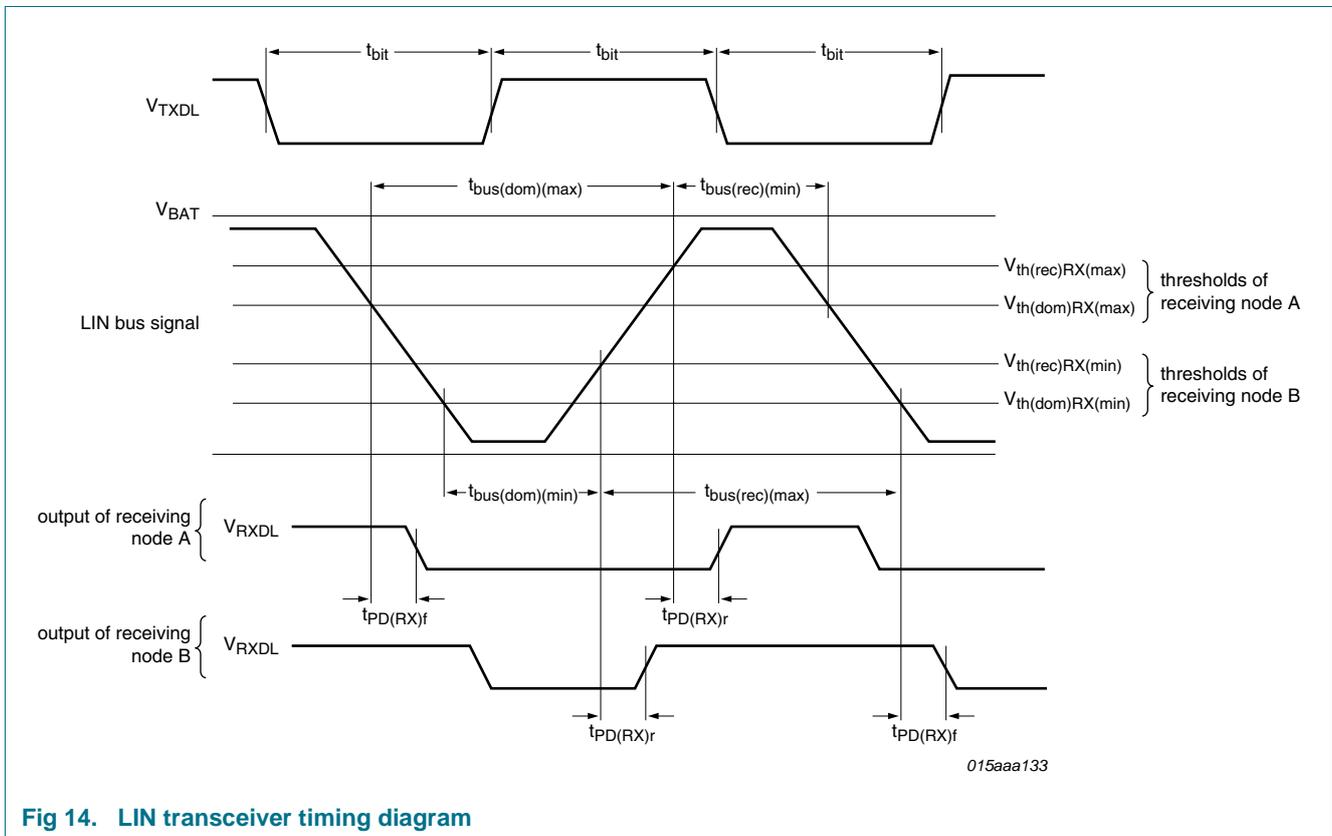
Fig 14. LIN transceiver timing diagram
