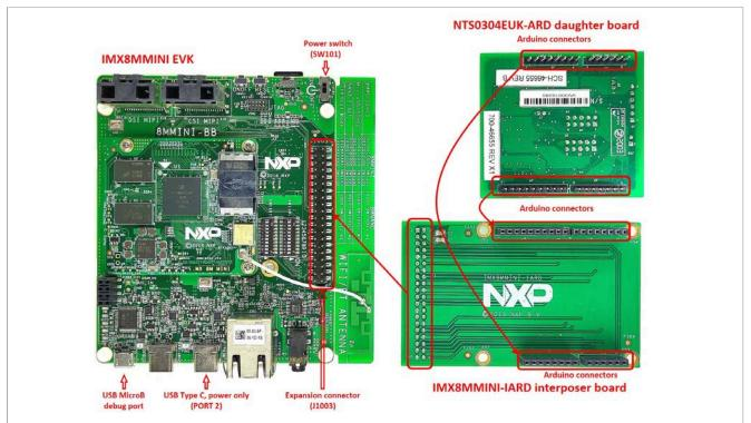
Figure 13. The assembly NTS0304EUK-ARD daughterboard, IMX8MMINI-IARD interposer board, and i.MX 8M Mini LPDDR4 EVK, before starting
