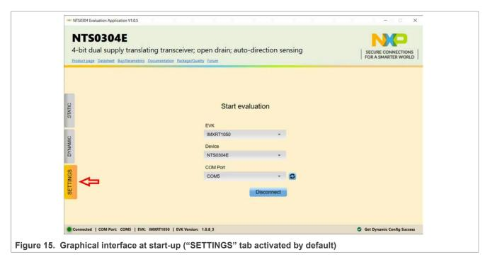
The GUI application starts with **SETTINGS** tab (marked with red arrow). The center of the window displays the board settings. The section provides the following settings:
