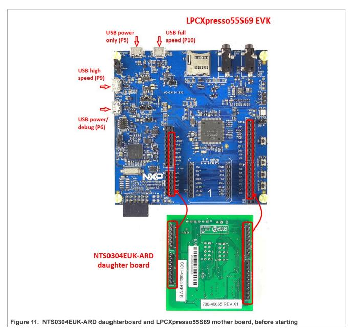
The following steps describe how to assemble, program, and operate the configuration shown in Figure 11.
