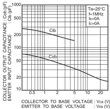
Fig.7 Collector output capacitance vs. collector-base voltage
