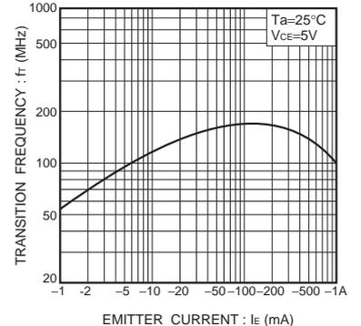
Fig.6 Transition frequency vs. emitter current
