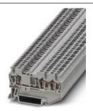
Feed-through terminal block, Connection method: Spring-cage connection, Cross section: 0.08 mm² - 1.5 mm², AWG: 28 - 16, Width: 4.2 mm, Color: orange, Mounting type: NS 35/7,5, NS 35/15
