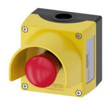
Enclosure for command devices, 22 mm, round, Enclosure material plastic, Enclosure top part yellow, with protective collar, 1 control point plastic, A=EMERGENCY STOP mushroom pushbutton red, 40 mm, rotate-to-unlatch, 1 NC, 1 NC, screw terminal, floor mounting, 1xM20 each on top and bottom
