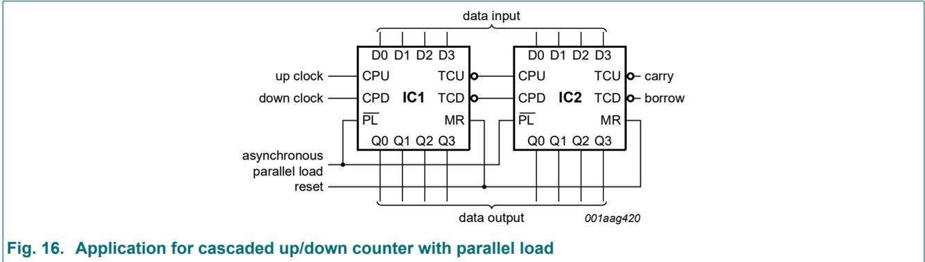
Fig. 16. Application for cascaded up/down counter with parallel load
