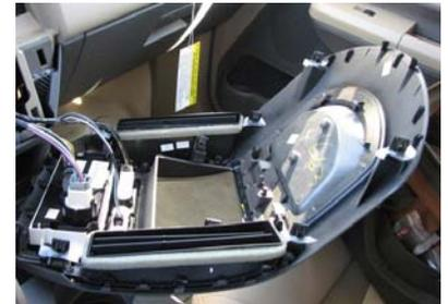
Radio Climate Control, Air Vent, Bezel Removed
