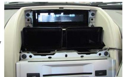
Air Vent Assembly Removed
