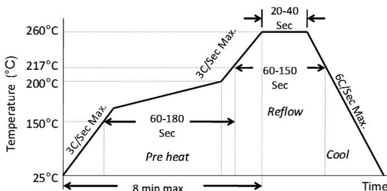
Figure 3. Solder Reflow Profile
