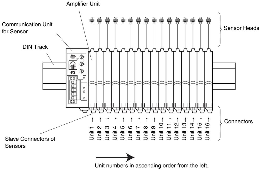
The Communication Unit identifies the connected Sensors according to the unit numbers. Unit numbers of sensors are assigned to the units from unit number 1 starting from the communication unit side. Note that some Sensors occupy two unit numbers.
