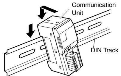
2. Press the rear part of the unit onto the DIN track.
