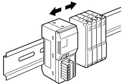
2. Keep pressing the communication unit in direction A and lift it up in direction B to remove.
