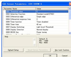
3) In the [Edit Sensor Parameters] dialog box, configure the following settings (depending on the fiber amplifier unit type, shown items vary):
