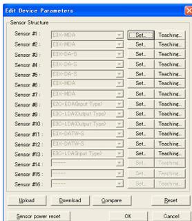
4. Click the [Set...] button on the right of the fiber amplifier unit type to monitor the current settings.
