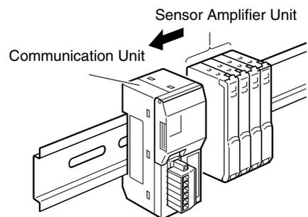
4. Fix the both ends firmly with End Plate (PFP-M, sold separately).
