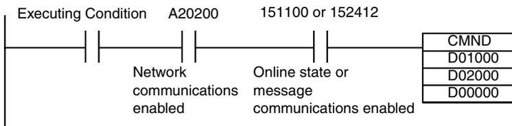
Command data of 10 bytes from D01000 is sent to destination node address 05, then its response data of 10 bytes is stored into D02000 of the local node (D00000 is control data)
