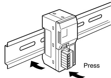
3. Slide the Sensor Amplifier Unit to fit the hook of the connector to the communication unit, and keep pushing until you hear it snap into place.
