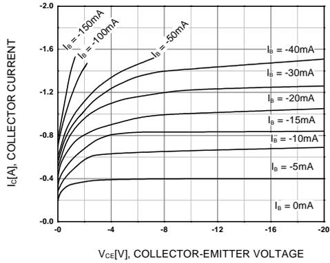
Figure 1. Static Characteristic
