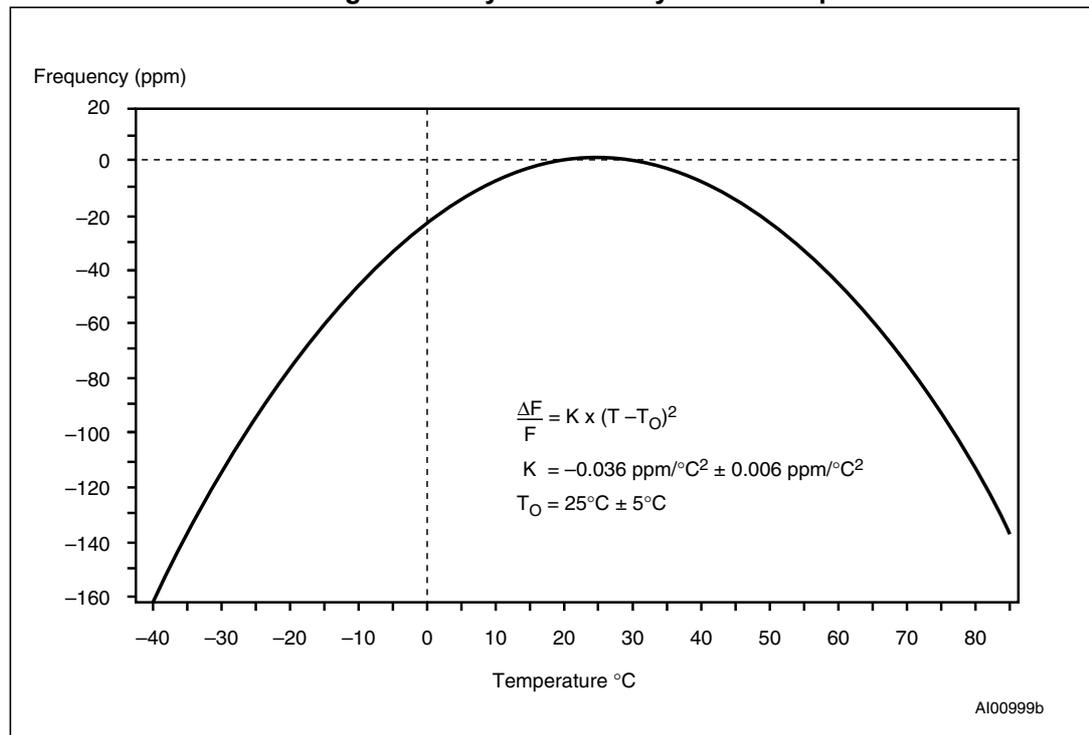
Figure 13. Clock calibration
