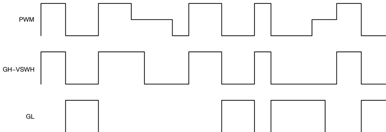
Figure 4. Timing Diagram
