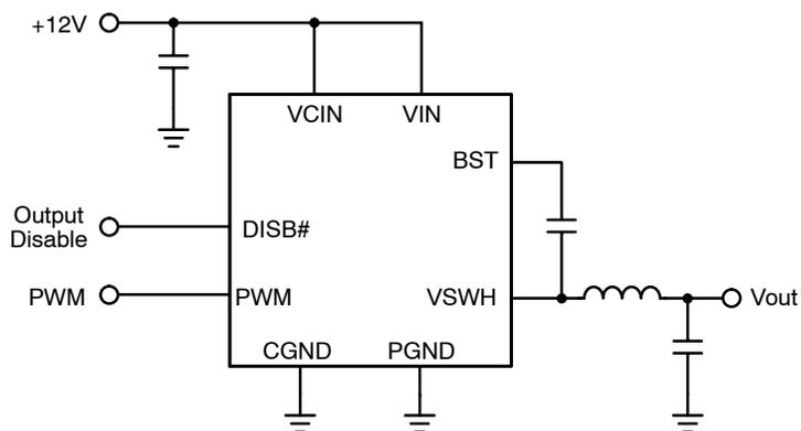
Figure 1. Application Schematic
