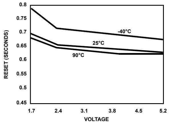
FIGURE 18.  $t_{WDO}$  VS. VOLTAGE/TEMPERATURE (WD1, 0 = 1, 0)
