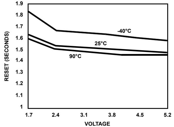
FIGURE 16.  $t_{WDO}$  VS. VOLTAGE/TEMPERATURE (WD1, 0 = 1, 1)
