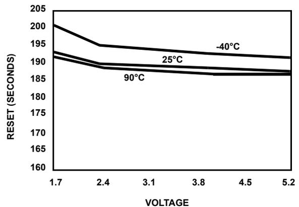
FIGURE 20.  $t_{WDO}$  VS. VOLTAGE/TEMPERATURE (WD1, 0 = 0, 1)
