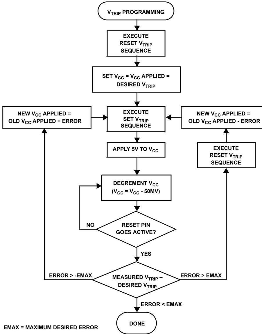
FIGURE 3. V<sub>TRIP</sub> PROGRAMMING SEQUENCE FLOW CHART
