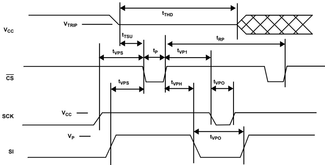
FIGURE 14.  $V_{TRIP}$  RESET CONDITIONS
