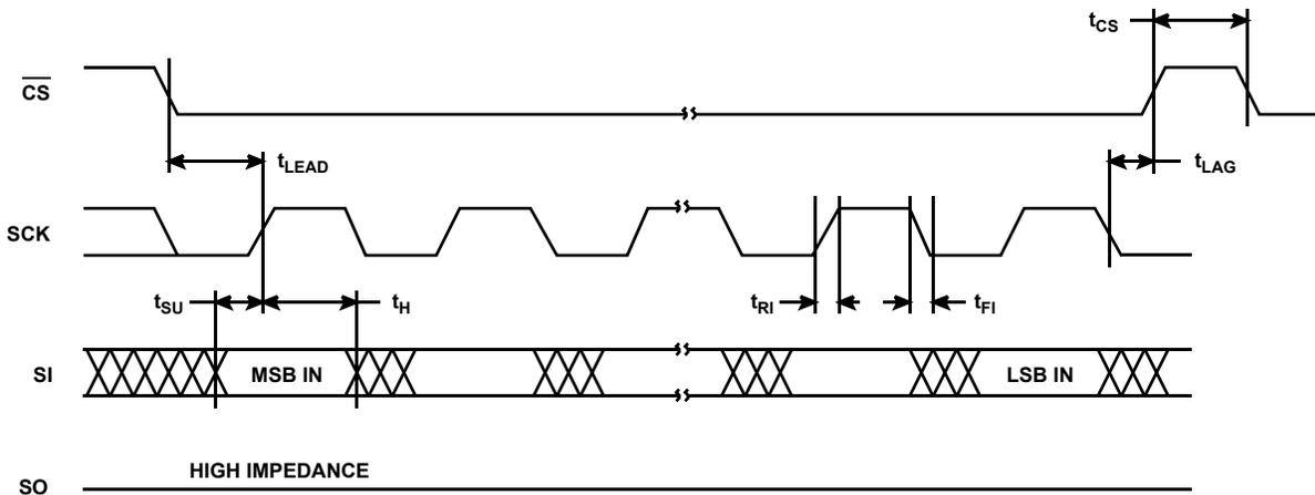
FIGURE 11. SERIAL INPUT TIMING
