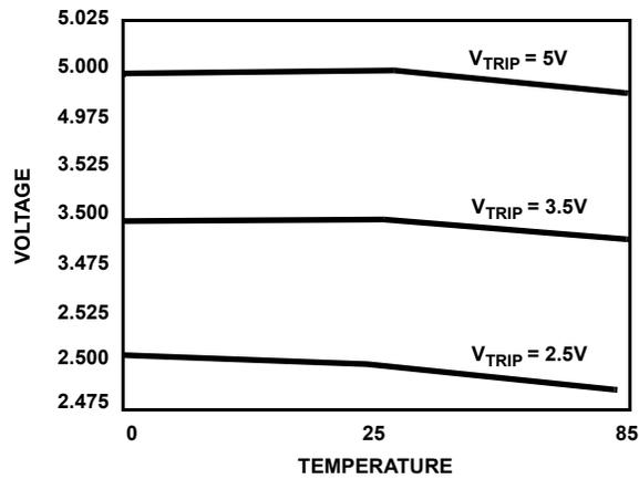
FIGURE 17.  $V_{TRIP}$  VS. Temperature (programmed at 25°C)
