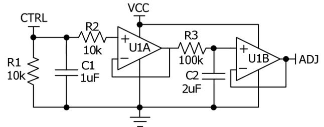
Figure 5. The Equivalent Circuit for CTRL Port
