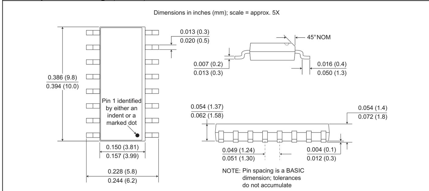
**0.3" 16-pin SOIC Package (no suffix)**
