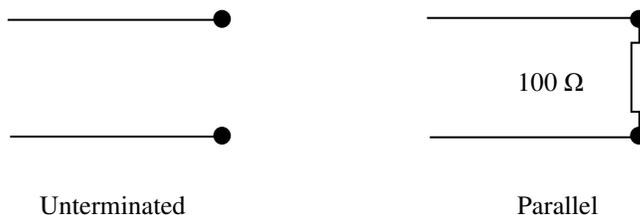
Proper termination is imperative when using IL3185 and IL3122 to minimize reflections. Unterminated lines are only suitable for very low data rates and very short cable runs, otherwise line reflections cause problems. Parallel terminations are the most popular. They allow high data rates and excellent signal quality.
