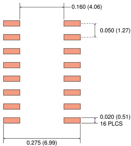
**0.3" 16-pin SOIC Pad Layout**
