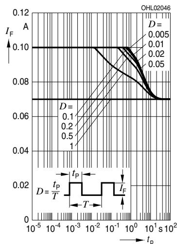
**Permissible Pulse Handling Capability****Zulässige Impulsbelastbarkeit  $I_F = f(t_p)$** D: Duty cycle,  $T_A = 85^\circ\text{C}$
