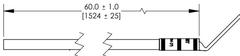
FACTORY CRIMPED #6 AWG COMMON BONDING NETWORK (CBN) JUMPER WIRE ASSEMBLY (QTY. 1) INCLUDES:
