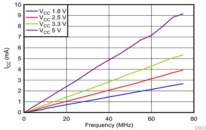
Figure 6. I<sub>CC</sub> vs Frequency
