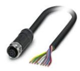
Sensor/actuator cable, 8-position, PE-X halogen-free, black-gray RAL 7021, free cable end, on Socket straight M12, A-coded, cable length: 2 m, for outdoor applications, with high-grade steel knurl
