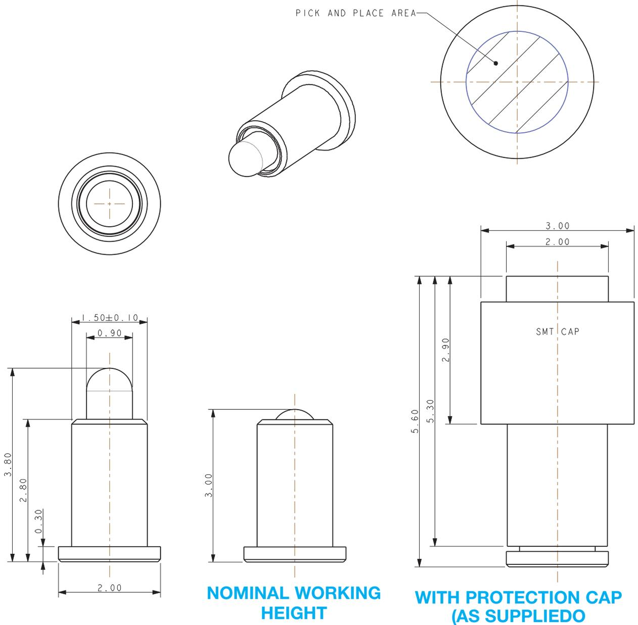
1. SERIES 9150 POGO PIN, WORKING HEIGHT 2.9MM TO 3.4MM.
