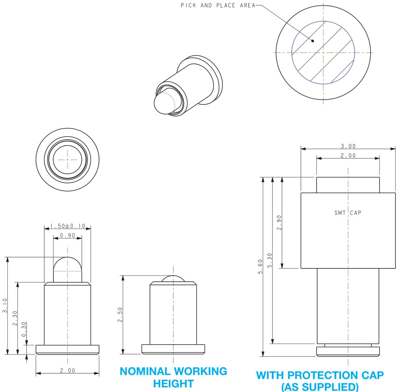
1. SERIES 9150 POGO PIN, WORKING HEIGHT 2.4MM TO 2.8MM.
